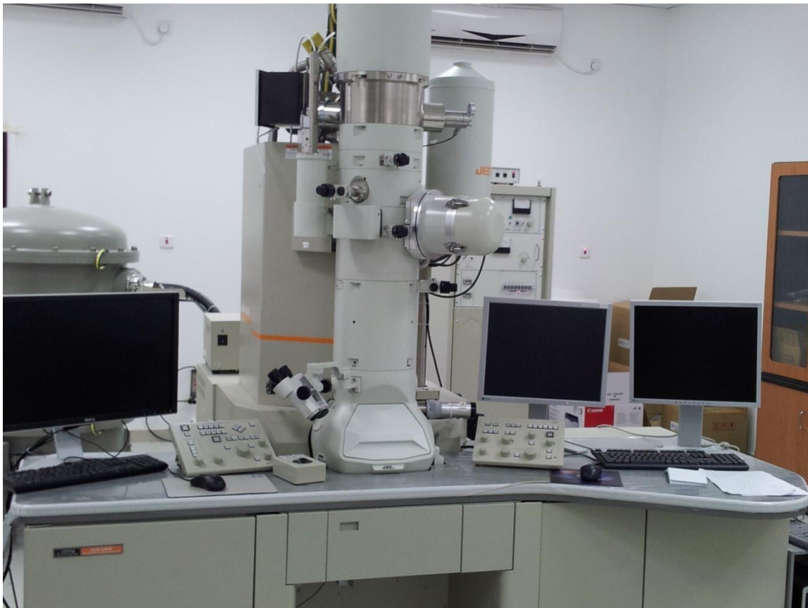
Figure 2.5. Schematic block diagram and real picture of high-resolution transmission electron microscope (TEM; JEM-2100F), based in Najran University Saudi Arabia
