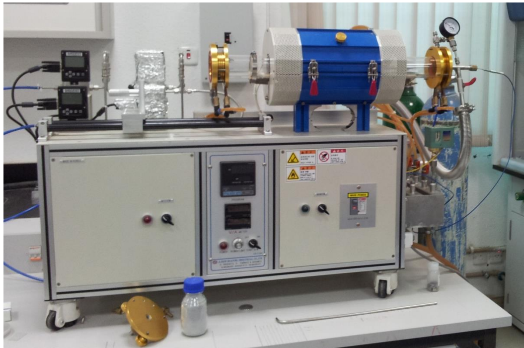
Figure 2.3. Schematic for the instrumental setup and real picture of the horizontal quartz tube furnace used for the growth of In-doped ZnO nanostructures, Ajeon Company, Korea based in Najran University Saudi Arabia
