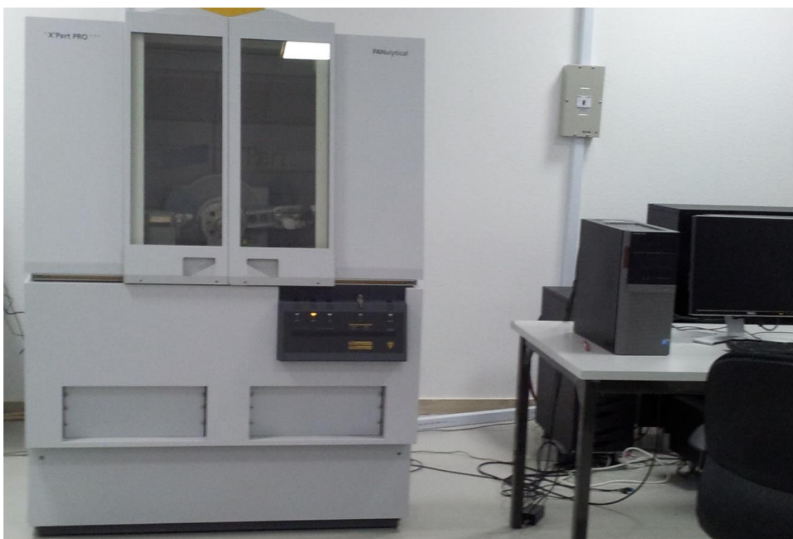
Figure 2.6. Typical block diagram and real picture of X-ray diffractometer (XRD; PANalytical Xpert Pro.) with Cu-K \alpha radiation ( \lambda=1.54178 \text{ \AA} ), based in Najran University Saudi Arabia
