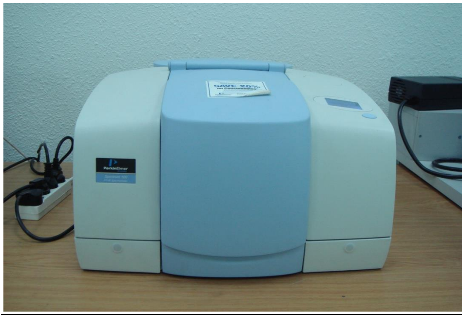
Figure 2.7. Real picture of Fourier transform Infrared spectrometer (FTIR; Perkin Elmer-FTIR Spectrum-100), based in Najran University Saudi Arabia
