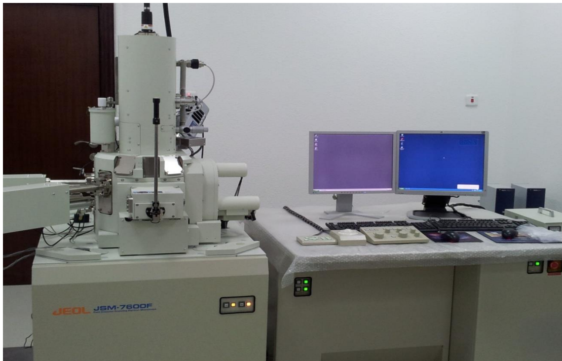
Figure 2.4. Schematic block diagram and real picture of field emission scanning electron microscope (FESEM; JEOL-JSM-7600F), based in Najran University Saudi Arabia
