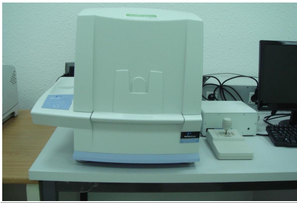
Figure 2.8. Real picture of Raman scattering spectrometer (Perkin Elmer-Raman Station 400 series), based in Najran University Saudi Arabia
