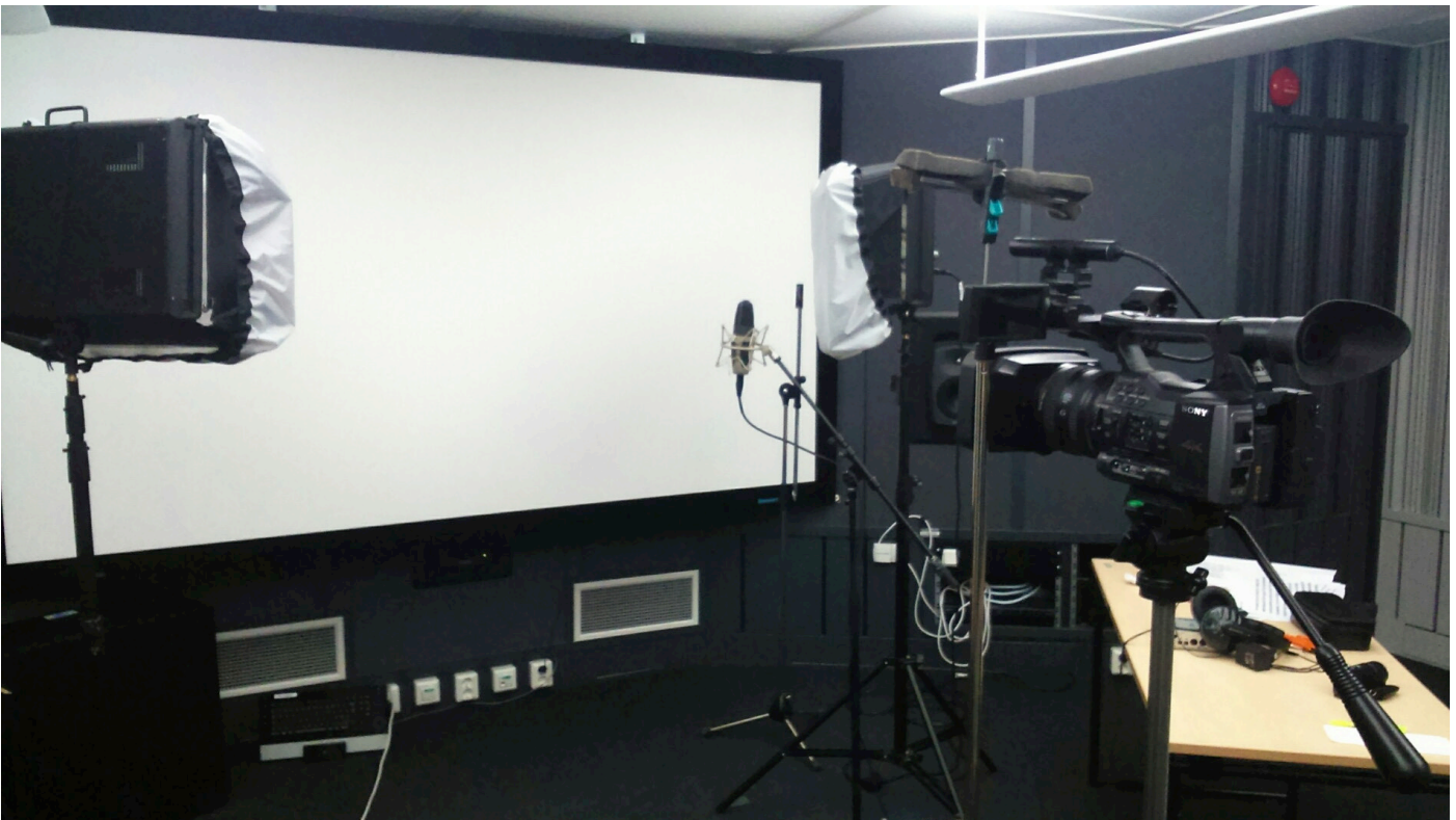
Figure 4. A closer look at the setup. The microphone is placed on the right hand side of the camera, pointing towards the middle of the screen.
