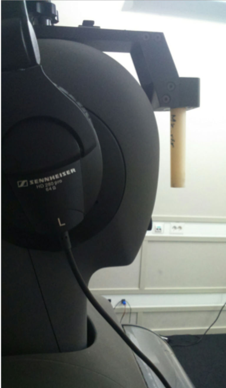
Figure 19. Sennheiser HD 280 headphones used for the test. The band of the headphones are adjustable for each person's own comfort. The picture is taken at Ericsson labs and modeled by an acoustic dummy head designed for recording binaural audio signals.
