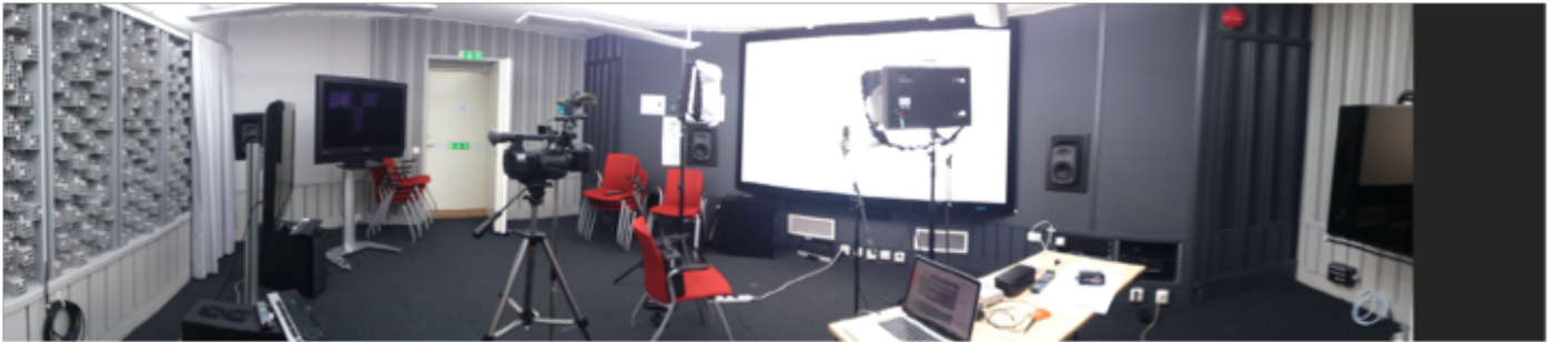
Figure 3. A snapshot of the equipment setup slightly before recording. The panorama picture reveals that the room has been treated with acoustic panels to minimize resonance and standing waves.
