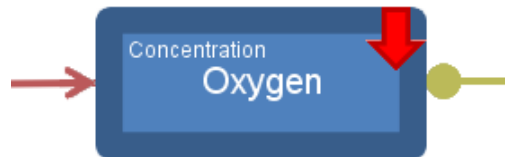
Figure 8: A node in a MILA model, representing the Concentration of Oxygen going down.
