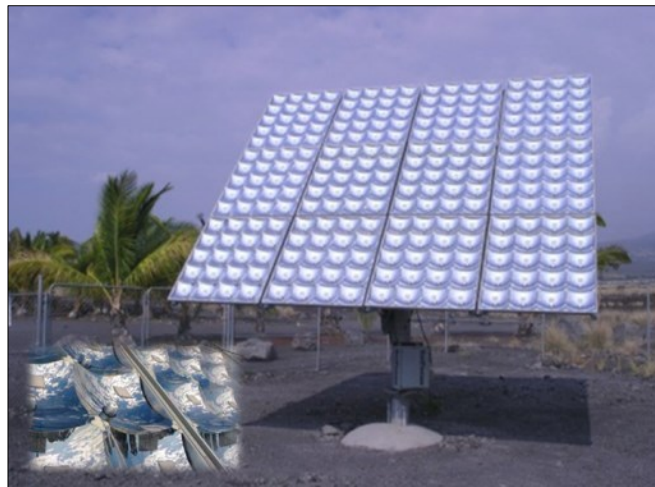
Figure 2-21: CPV demonstrator developed by Solfocus, deployed in Kailua Kona at the National Energy Laboratory of Hawaii [15, 47, 49].
