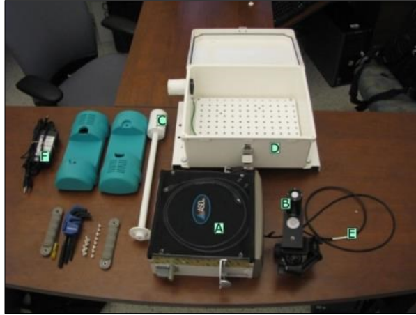
Figure 3-17: Parts of the spectroradiometer setup on the tracker at the site. The spectroradiometer from Figure 3-15 has been partially disassembled to fit into an environment controlled housing. (A) The spectroradiometer; (B) The cosine receptor; (C) The direct attachment; (D) The housing for mounting the spectroradiometer; (E) A flexible fiber optic cable which connects the spectroradiometer to the cosine receptor. Adapted from [15].
