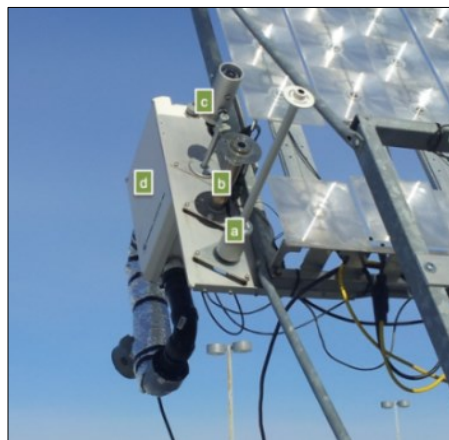
Figure 3-16: Instrument panel on a tracker at the APECS test site. (a) Spectroradiometer attachment. (b) Eppley NIP pyrheliometer; (c) CCD camera and (d) temperature controlled ASDi housing for spectroradiometer environmental stabilization.
