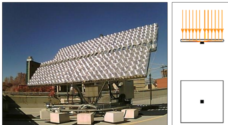
Figure 2-16: The APECS demonstrator at the University of Ottawa solar test site (Left). An illustration of the light guide optics used to concentrate sunlight on the multi-junction cell (Right).
