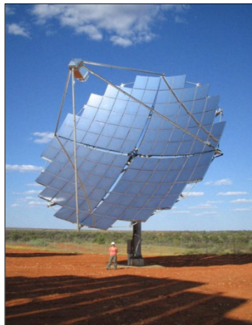
Figure 2-18: A parabolic light concentrating dish using mirrors at the Hermannsburg power station in Australia [15, 45].
