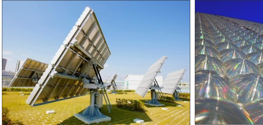
Figure 2-20: Dome shaped Fresnel lenses concentrating systems. [44].
