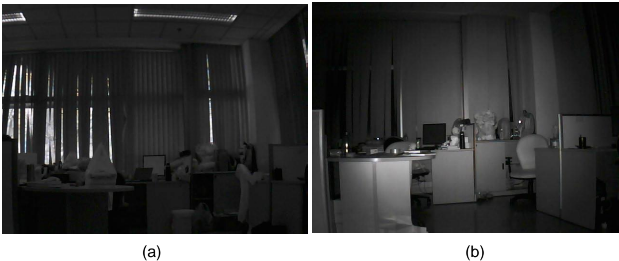
Figure 24: Imaging results using HWB 830 filter, (a) taken in the day time, (b) taken in the night with self infrared lighting from the camera
