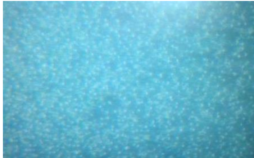
Figure 30: Unexpected light dots on top of the surface of the substrate with coating
