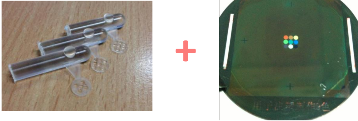
Figure 53: Comparison sample, ACE structure made by injection molding + pigment based photoresist multi-spectra filter
