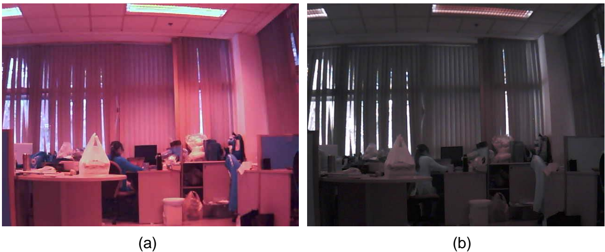
Figure 23: Red glass filter images, (a) HB630 result images; (b) HB700 results images
