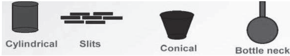
Figure 23 Different pore shapes in activated carbon [103]
