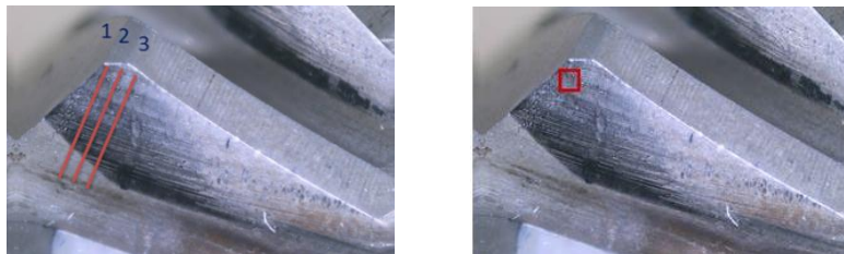
Figure 26. On the left the 3lines 2D measurement of the 1 st repetitions, on the right the square area of 0.5x0.5 mm
