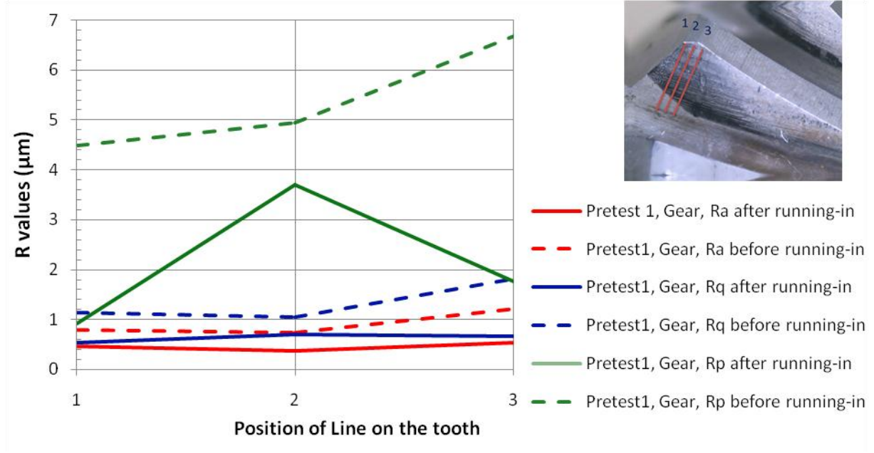
Figure 41. Roughness values on gear tooth, pretest 1 . Horizontal axis is presenting the position of 2D measurement on the gear flank and vertical axis is presenting R_a , R_q and R_p values in \mu\text{m} .
