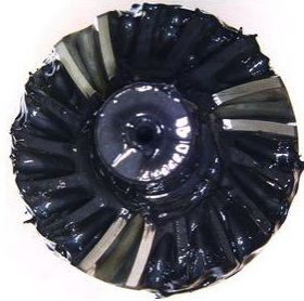
Figure 24. A gear which is ready for 2D roughness measurement.
