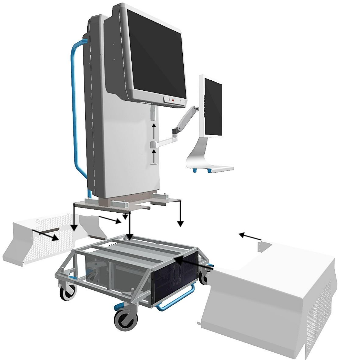
Figure 52. The four main modules of the demo-workstation are the 3D screen body, the 2D screen and arm, the aluminum frame base and PC and lastly the base covers. The modules are assembled as shown in the figure.
