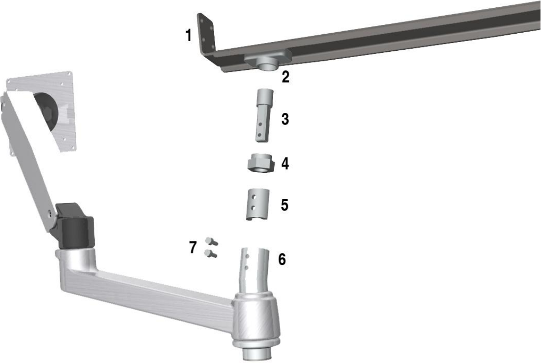
Figure 37. 2D monitor mounting bracket components: 1. Sheet metal support structure, 2-4. Current mounting brackets for the mouse- and keyboard tray, 5-7. Adaptor parts enabling attachment of the LX Desk Mount LCD Arm.
