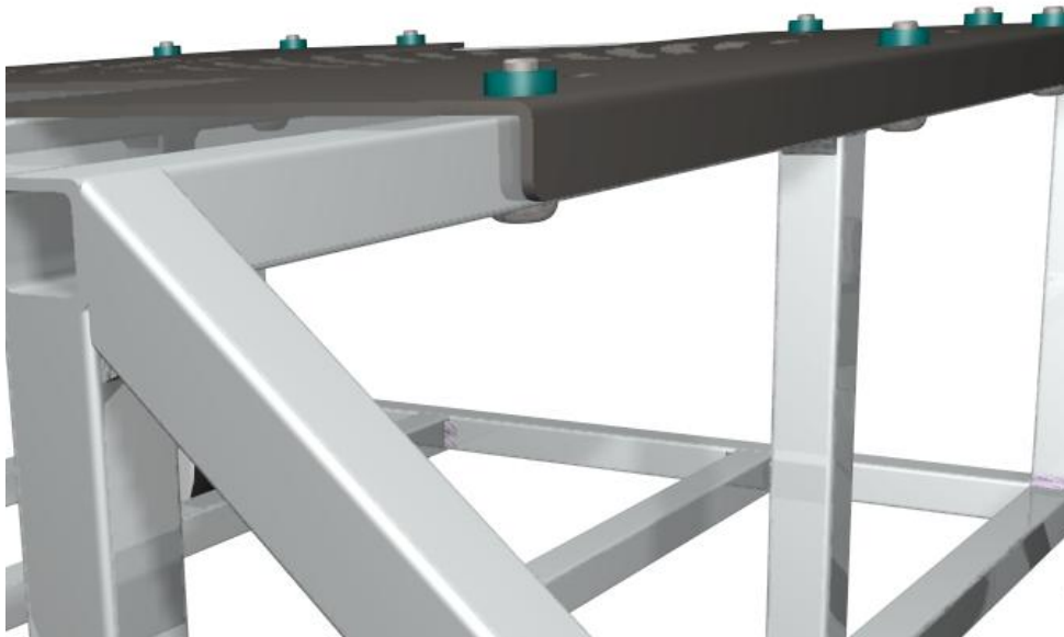
Figure 28. The base plate is fastened to the aluminum frame using ten M8 screws that fit the clinch nuts that are fixed to the base plate.
