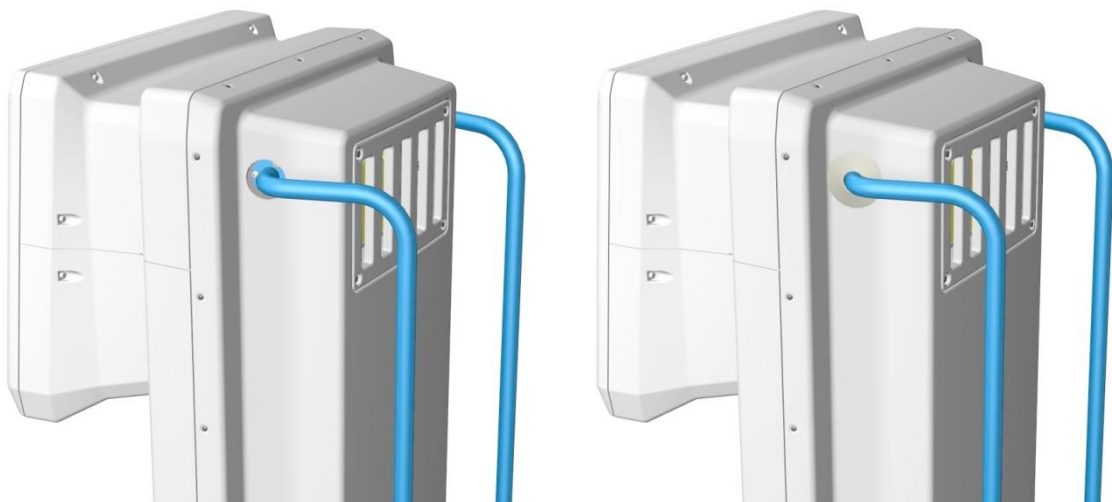
Figure 34. The left image shows the hole that is cut in the rear cover in order to fit the handle. The image to the right shows the same image but now with the rubber gasket that covers the hole in place.
