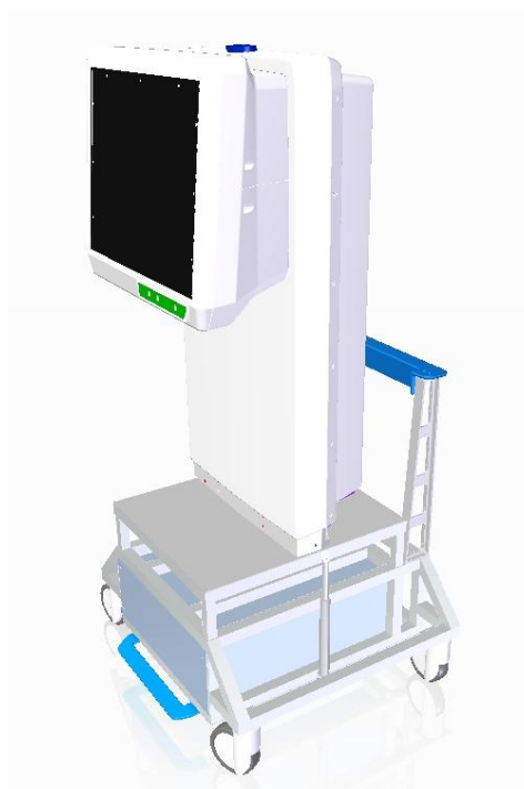
Figure 20. Concept 2 with a height adjustable base plate controlled by gas dampers.
