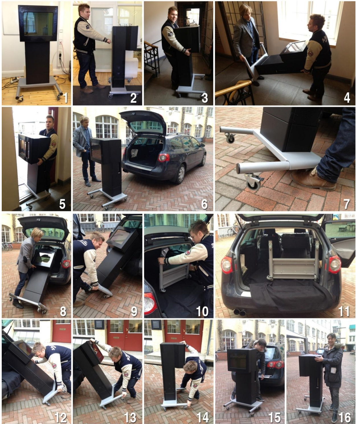
Figure 8. Steps involved in transporting the MD-20 workstation from the office to the car, loading it into the car and unloading it from the car.
