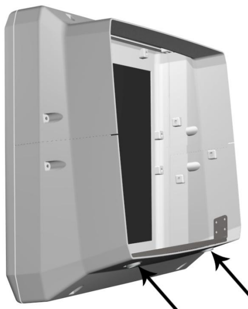
Figure 36. Mounting brackets attached to the support structure on the inside of the 3D screen’s casing. The brackets go through two holes in the casing, making it accessible from the outside.
