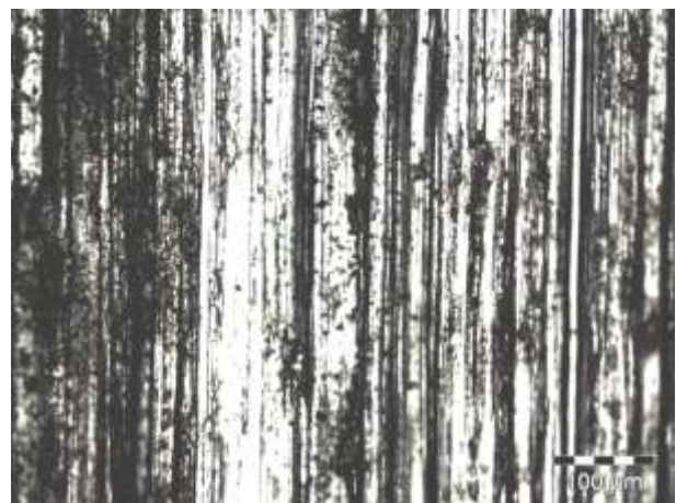
Figure 4.16: Microscope images of the Ti6Al4V pin couple on Ti6Al4V with a normal force of 10N; a) 100X MAG, b) 200X MAG
