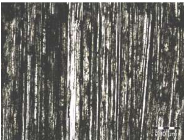
Figure 4.16: Microscope images of the Ti6Al4V pin couple on Ti6Al4V with a normal force of 10N; a) 100X MAG, b) 200X MAG
