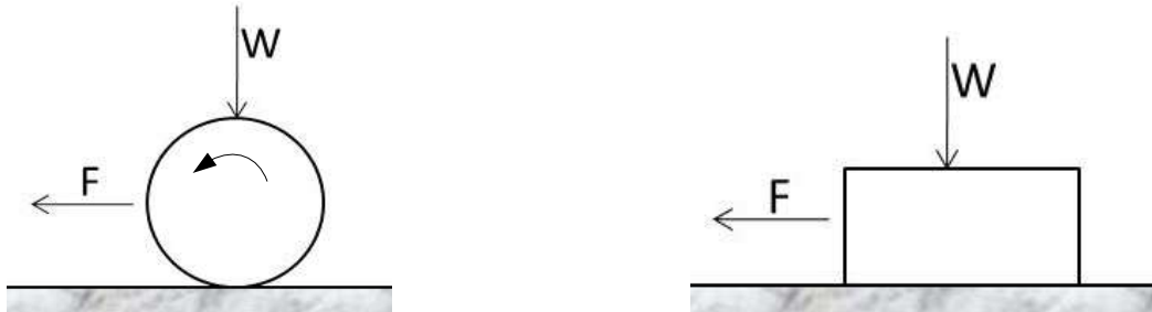
Figure 2.1: Illustrations of a rolling contact and a sliding contact with frictional force F (adapted from [2,21])
