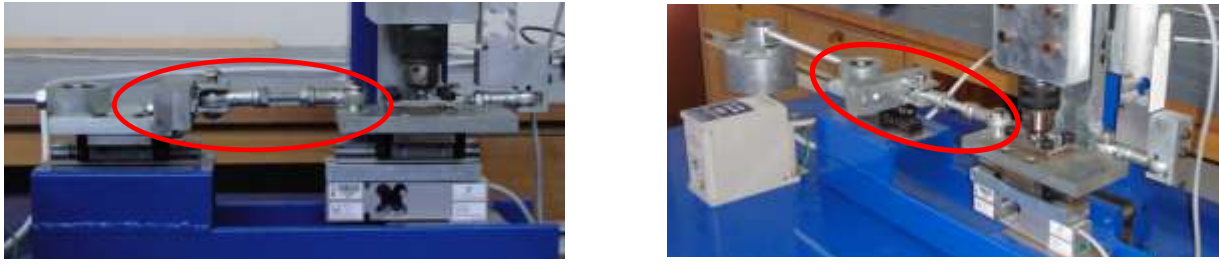
Figure 3.7: Image depicting the new linkage
