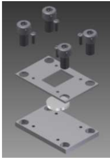
Figure 3.10: Exploded CAD view of the clamp system for the flat specimen
