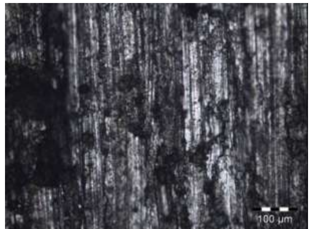
Figure A.2: Microscope images of the Ti6Al4V pin couple on Ti6Al4V with a normal force of 50N; a) 100X MAG, b) 200X MAG
