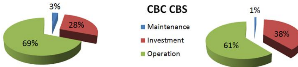
Figure 33: The total life cycle cost of the CBC system (left) and the CBS system (right)
