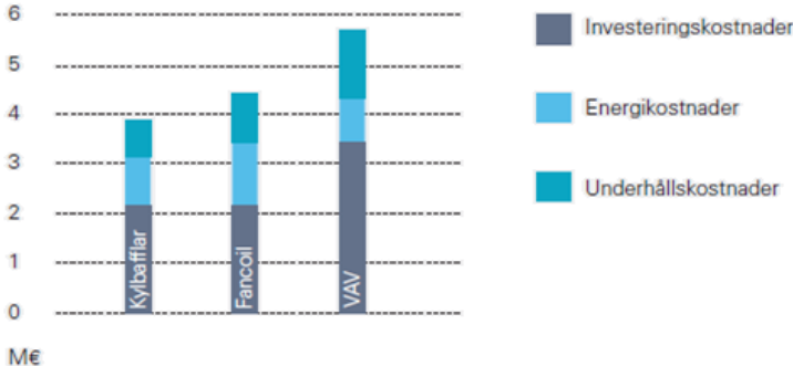
Figure 35: Life cycle cost for Halton cooling beams (left) according to Olof Granlund Oy
