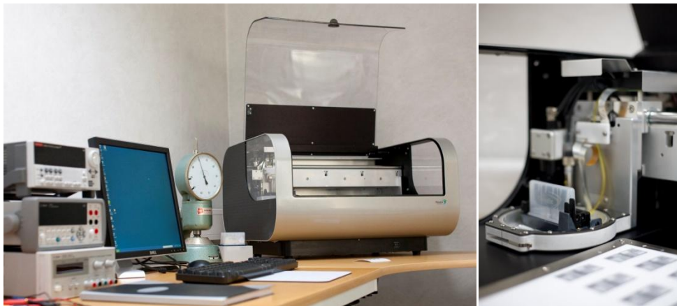
Figure 1. The piezoelectric functional materials inkjet printer used during the work of this thesis.
