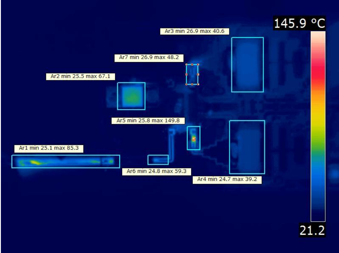
Figure 72. IR picture taken at 200 watts of forward power.
