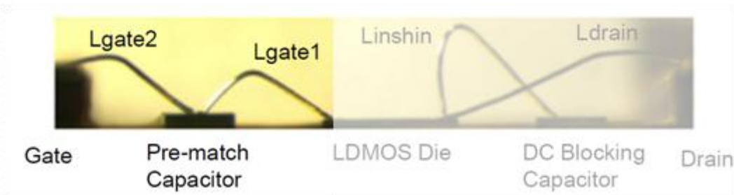
Figure 5. Side- view picture of a transistor with conventional matching at both side [2].
