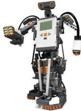
Figure 7 Lego Mindstorms. In the center, the body of the robot is the programmable intelligent brick.
