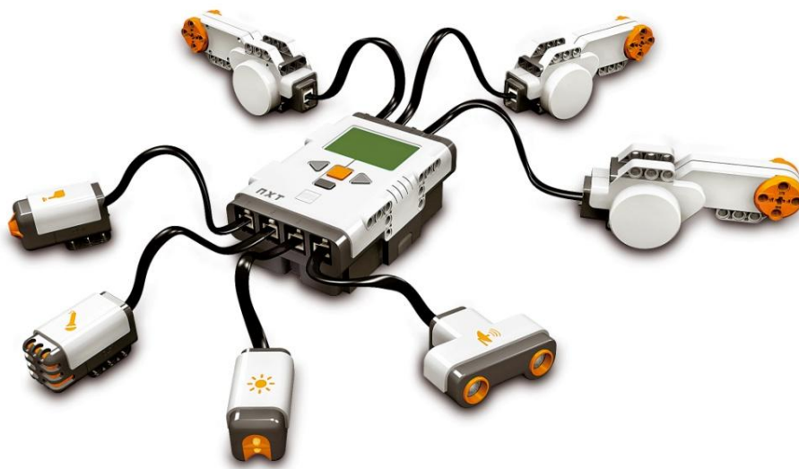
Figure 6The NXT Intelligent Brick (in the middle) and the three motors, the four standard sensors.
