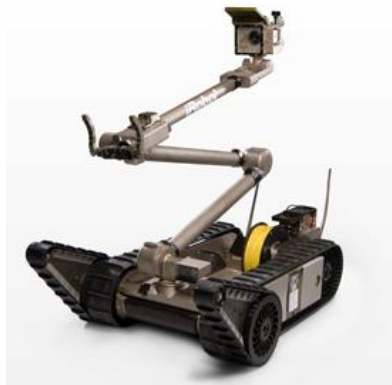
Figure 5 Robot from Fukushima, designed to clean up in the nuclear power plant.
