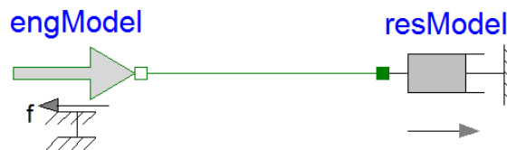
Figure 3.1: The icon view , of the Vehicle -model. Consisting of an engine component connected to a resistance component.
