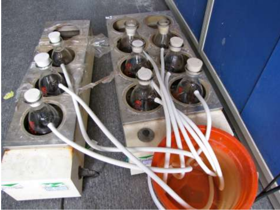
Picture 4.1, 9 bottles sealed with a rubber plug and with gas outlet in a bucket of water
