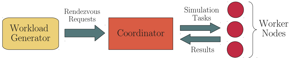
Figure 3.1: Distributed rendezvous simulator architecture
