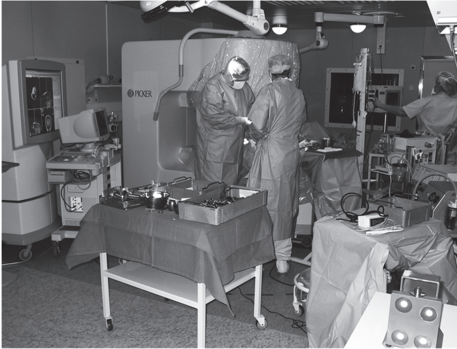
Fig. 1. The Proview scanner was a C-shaped iron core electromagnet with a 44 cm patient gap. The advantages of the scanner included the possibility to turn it off, with a 6-minute ramp to imaging time, and a fully detachable patient couch that was movable on rails. Neurosurgical tumor resection was performed outside the MR scanner. Use of non-MRI-compatible instruments and devices (such as the ultrasound scanner, left) during a neurosurgical operation was rendered possible by the resistive magnet's turn-off feature. One fiber optic and two single surgical lights, four anesthesia gas inlets, 48 sockets and filtered air ventilation complete the operating room environment.
