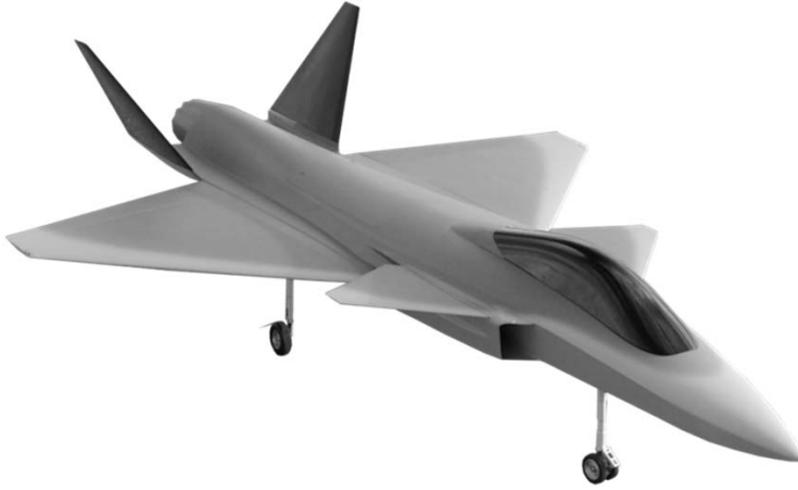
Figure X.13 The sub-scale RC prototype of the GFF ready for its maiden flight [III]
