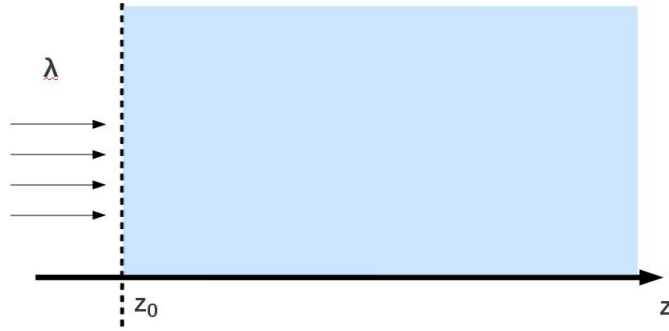
Figure 2.1: Interface between a dielectric and an absorber material ( z \geq z_0 ). The light is propagating from left to right along z -axis.
