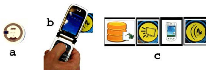
Fig 8. The MEDUSA composition tool: (a) A sticker with NFC tag, (b) an NFC-enabled mobile phone, and (c) example service cards. (VIII, ©2011 IGI Global. Reprinted by permission of the publisher).
