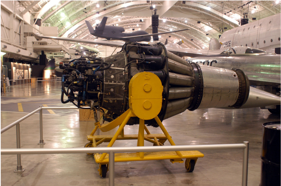
Figure 1.1. Allison J33 turbojet engine with centrifugal compressor and can combustors.
