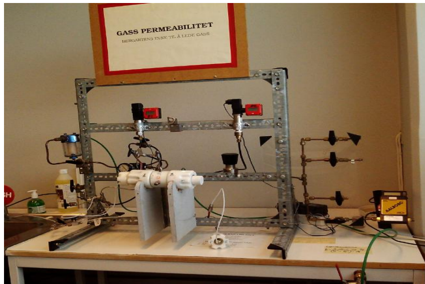
Figure 3.6: Shows the Constant Head Permeameter apparatus used to measuring pressures ( P_1 ) and ( P_2 ) and air flow rate.
