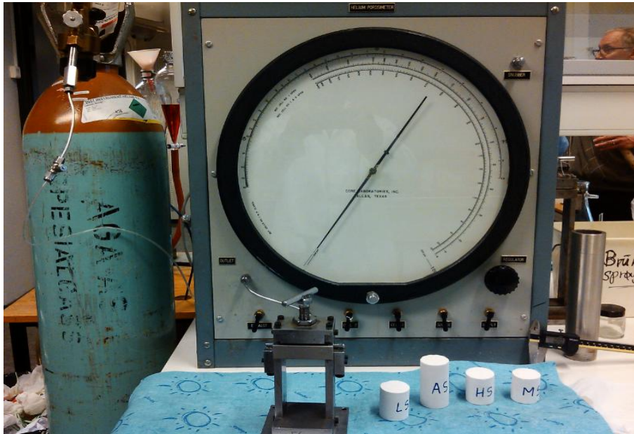
Figure 3.5: Shows the Helium porosimeter apparatus (Core Laboratories, Inc.) used for measurements of the volumes V_1 and V_2 .
