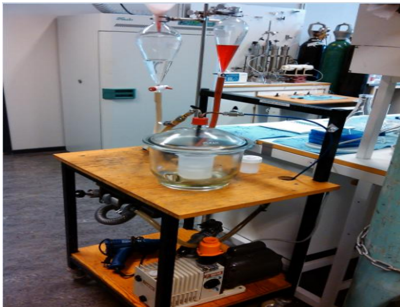
Figure 3.7: Shows the vacuum Eksikotor (extractor) apparatus used for core saturation.
