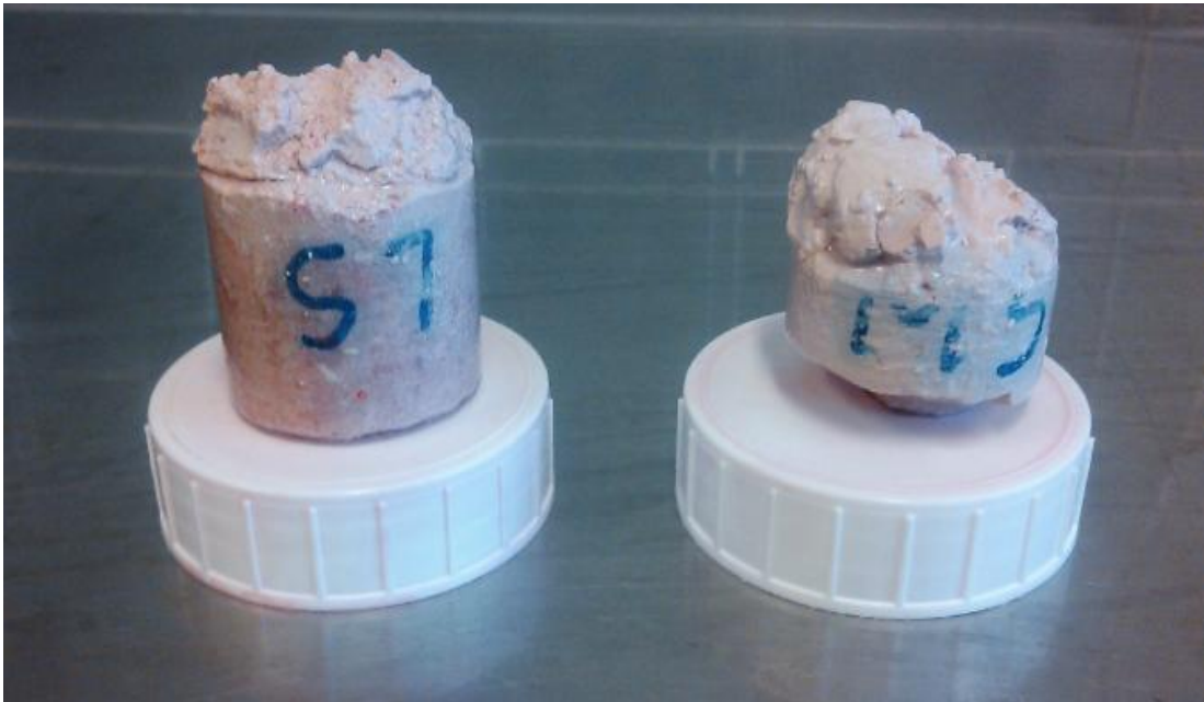
Figure 4.7: Shows the samples LS and MS damaged after( imbibition) water flooding process.
