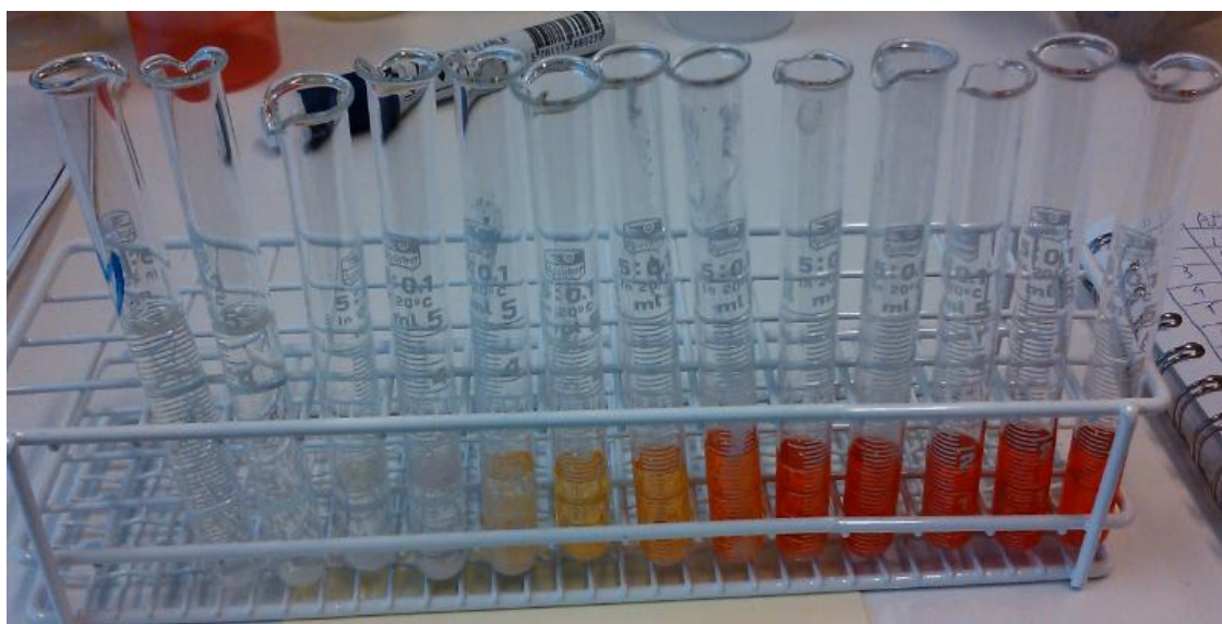
Figure 4.4: Shows the results of oil production in tube of core MS after drainage.
