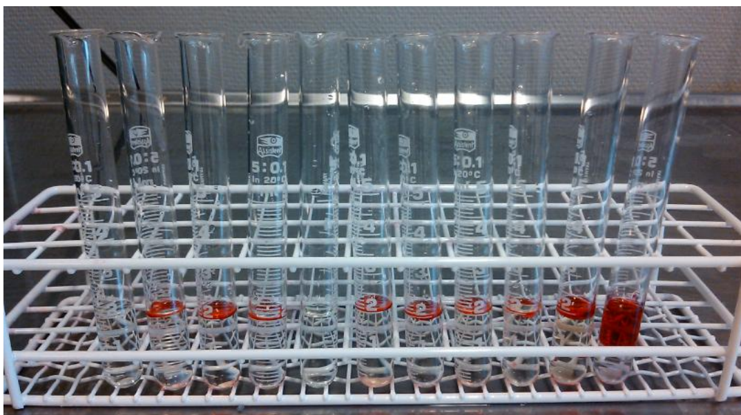
Figure 4.9: Shows the results of oil production in tube of core CS after imbibition.
