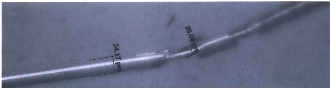
Figure 5. Optical micrograph of microwire with and without its glass coating
