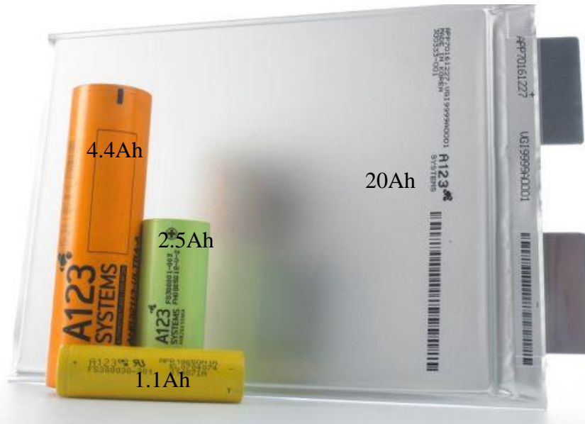
Figure 2. A variety of cells from manufacturer A123 System including three cylindrical cells and one pouch. Picture is courtesy of http://www.a123systems.com
