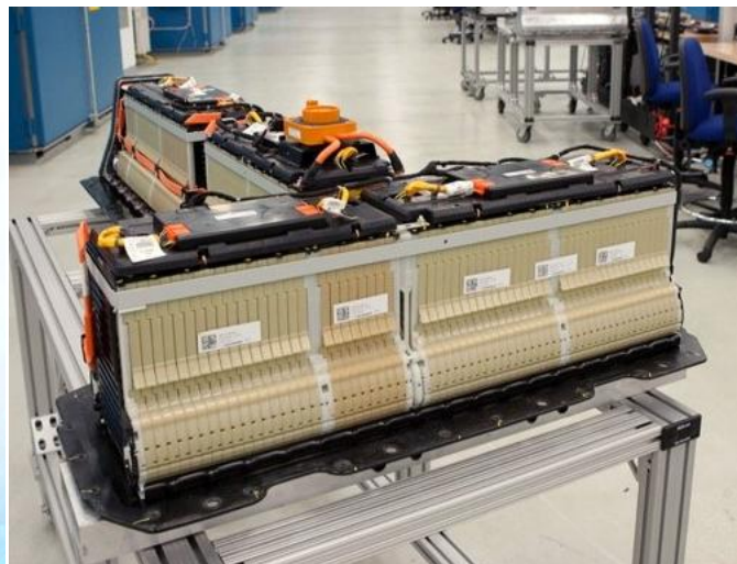
Figure 3. ESS that is used in Chevrolet Volt from General Motors is built up from cells arranged in modules. Picture courtesy of www.gm.com and www.gm-volt.com
