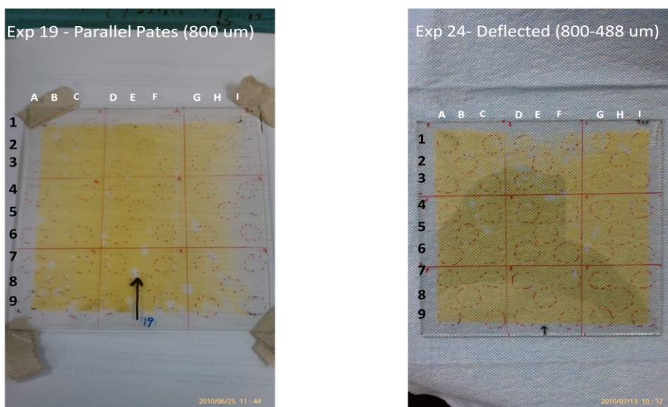
Figure 4-4: Labeling system for measuring points (left) Parallel plates (right) Deflected plates.
