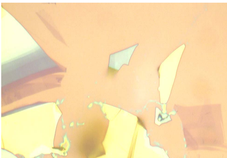
Figure 12. Optical microscope image of FLG obtained by micro-mechanical cleavage.
