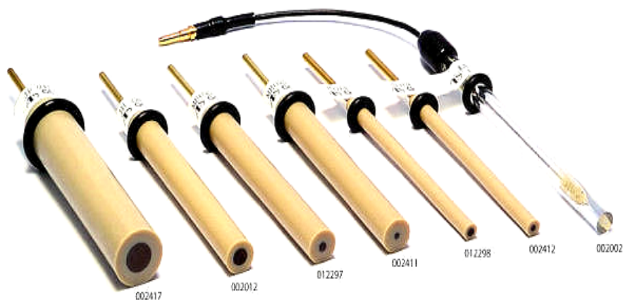
Figure 15: Illustration of the different types and sizes of glassy carbon electrodes (GCE) [146]
