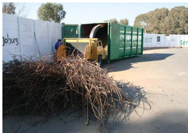
Photograph 3.7: Shredding of waste before loading
