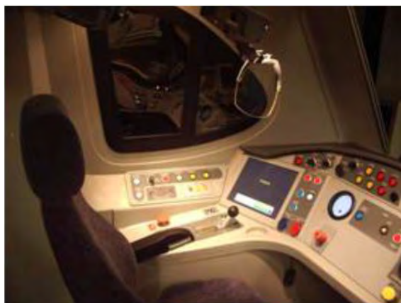
FIGURE 1 HUD fitted to a full-task train simulator.
