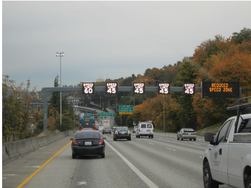
Figure 70. CMS near Seattle indicating current managed lane speed limit different from general-purpose lanes.
