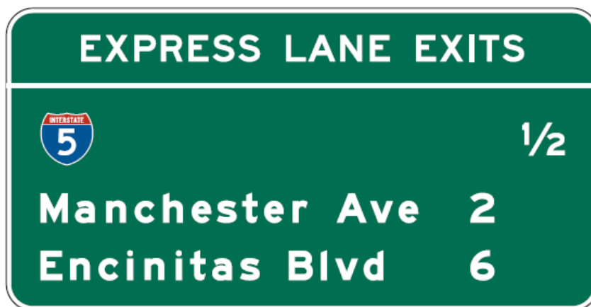
Figure 69. MUTCD Figure 2G-19 example of an exit destination sign for a managed lane.
