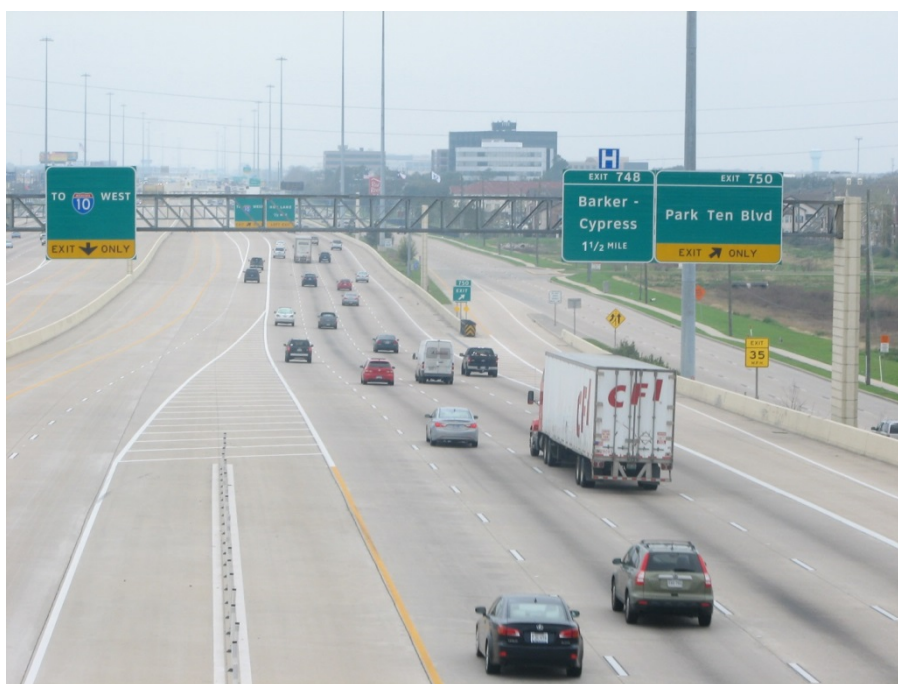
Figure 51. Exit from managed lane using an auxiliary lane on the Katy Freeway (I-10) in Houston, Texas.
