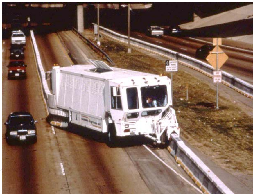
Figure 77. Deployment of contraflow lanes by moveable barrier.
