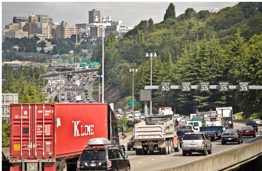
Figure 26. Dynamic speed signs in Seattle (HOV lane is leftmost with higher speed).
