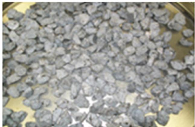
Manually separated No. 6 Stone with limited evidence of RAP binder transfer
