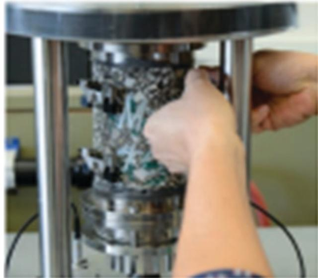
FIGURE 15 Simplified viscoelastic continuum damage set up (Source: NCHRP 9-57 Workshop 2015).
