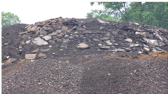
FIGURE 18 Example of RAP from variations in RAP materials from various sources [demolition (*top, center*) and millings from different projects (*bottom*)] (Source: West 2010).
