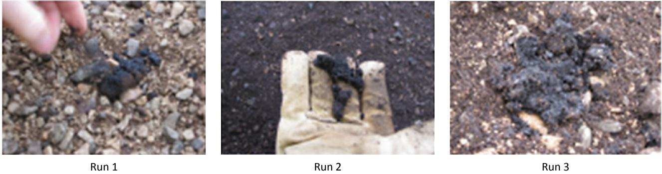
FIGURE 40 Balls of asphalt and fines after dry mixing in batch plant (no virgin asphalt) (Source: Johnson et al. 2013).
