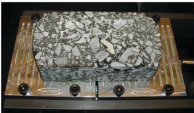
FIGURE 12 Overlay tester for evaluating reflective cracking resistance (Source: Klutzz and Mogawer 2012).
