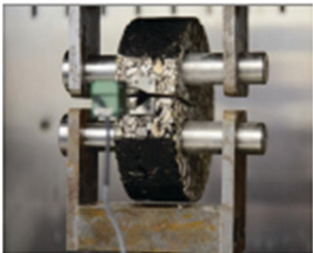
FIGURE 10 Disc-shaped tension test (Source: NCHRP 9-57 Workshop 2015).
