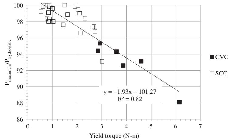
(b) Ratio of  $P_{\text{maximum}}/P_{\text{hydrostatic}}$  versus yield torque.
