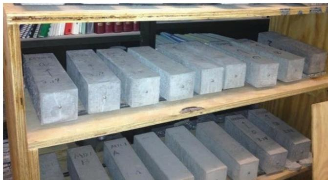
**Figure 1-11. Drying shrinkage specimens.**
