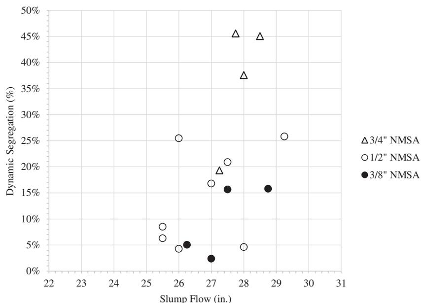
Figure 2-8. Flow trough dynamic segregation versus slump flow.
