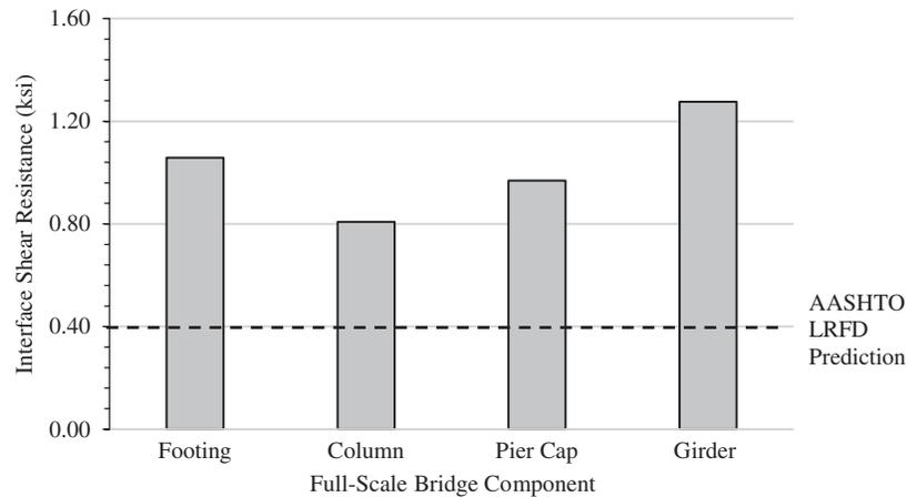
**Figure 2-25. Interface shear resistance of unreinforced SCC push-off specimens.**
