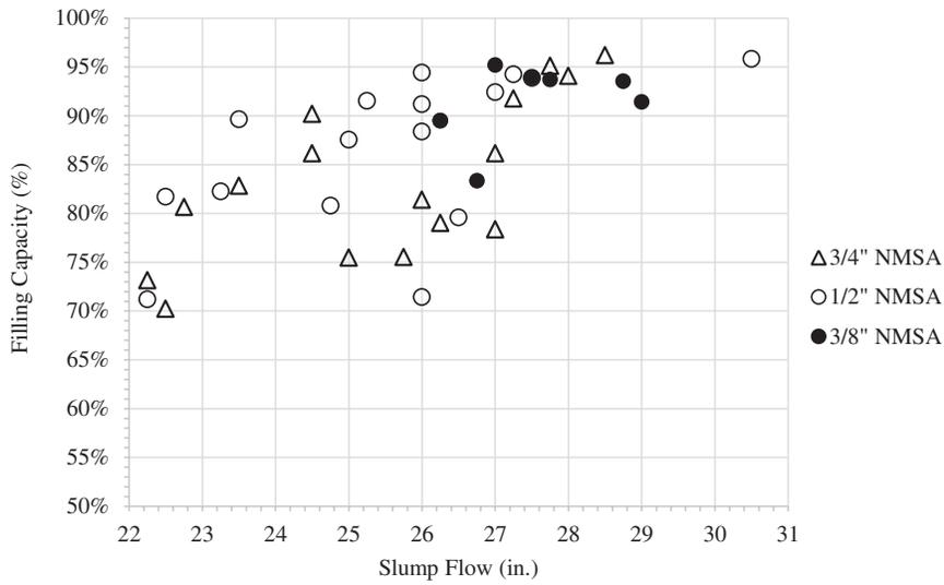
Figure 2-5. Caisson filling capacity of SCC versus slump flow.
