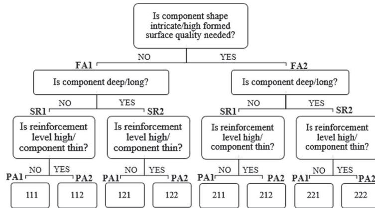
Figure 1-3. Process for determining workability targets.
