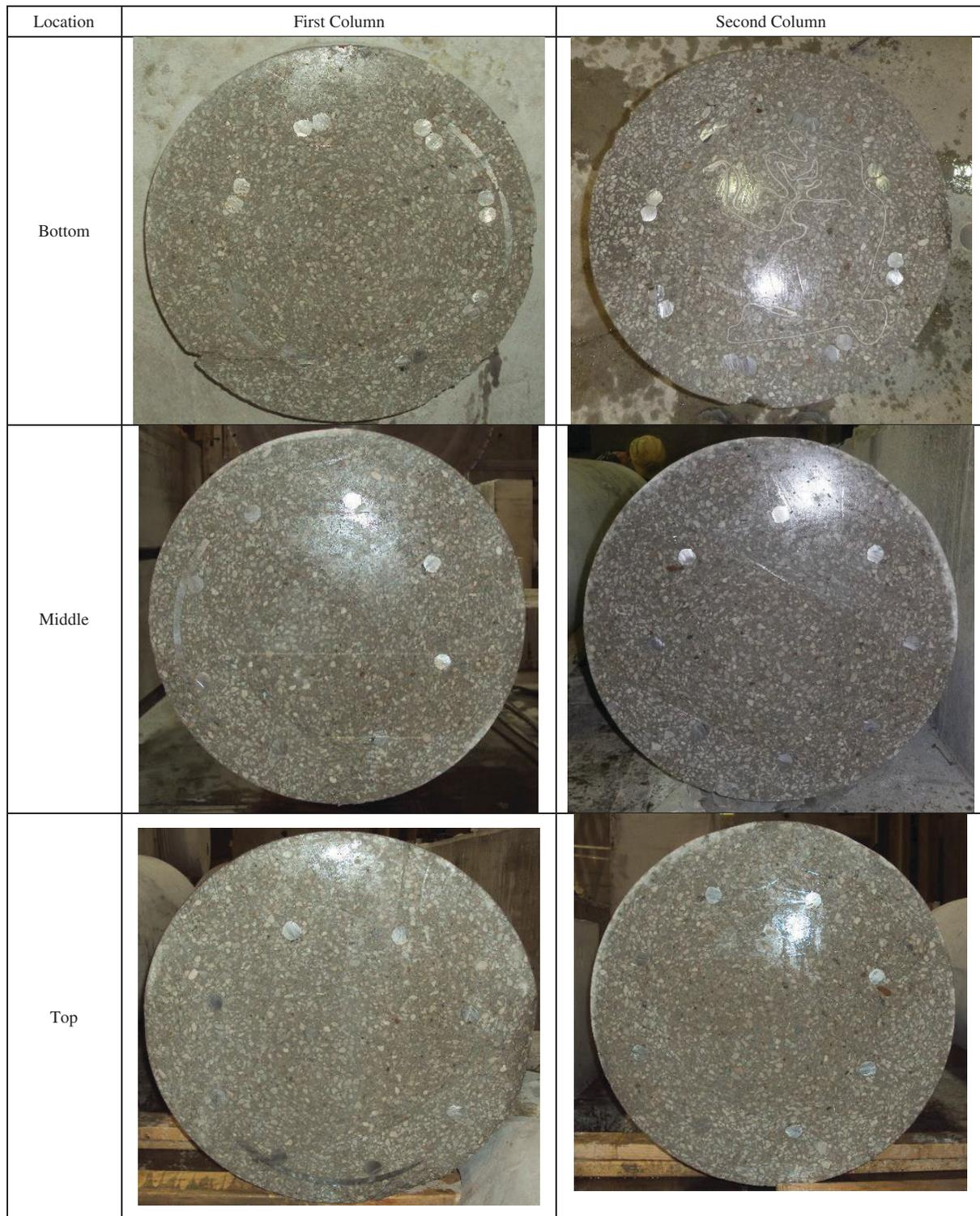
**Figure 2-41.** Saw cuts at the bottom, middle, and top of the two pier columns.
