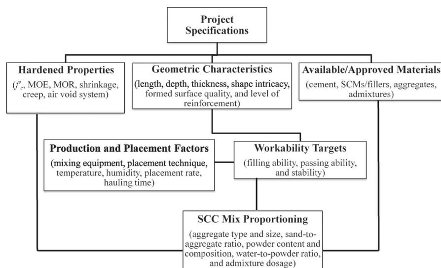
Figure B-1. General steps of proportioning SCC mix for cast-in-place bridge components.
