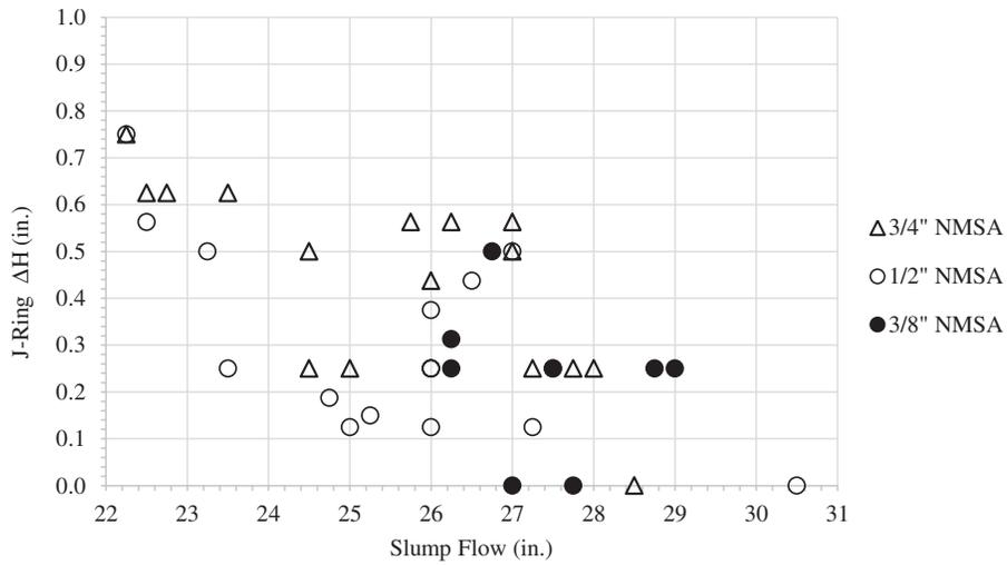
Figure 2-4. J-ring difference in average height ( $\Delta H$ ) versus slump flow.
