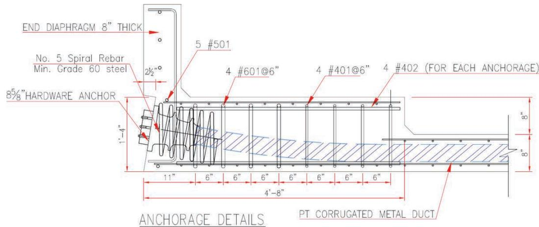
Figure 1-17. Reinforcement details of the box girder specimen.
