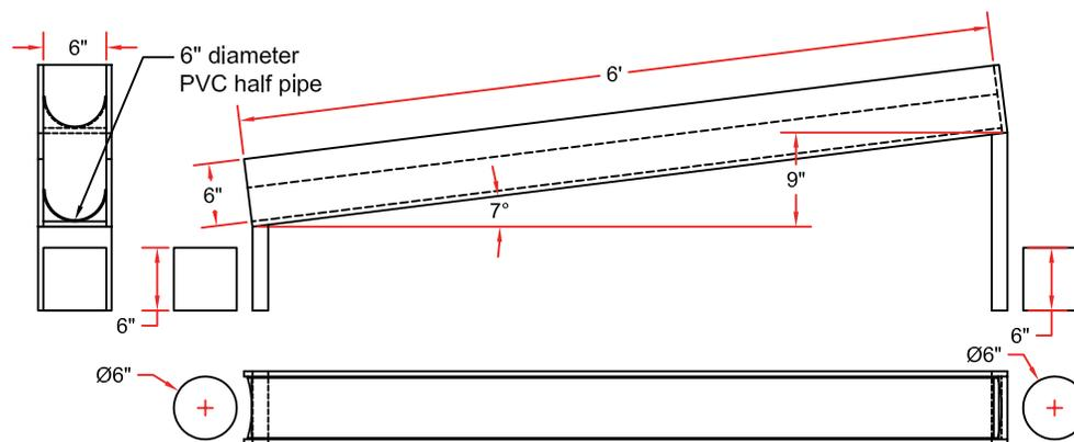
**Figure 1-5. Modified flow trough used for evaluating dynamic stability.**
