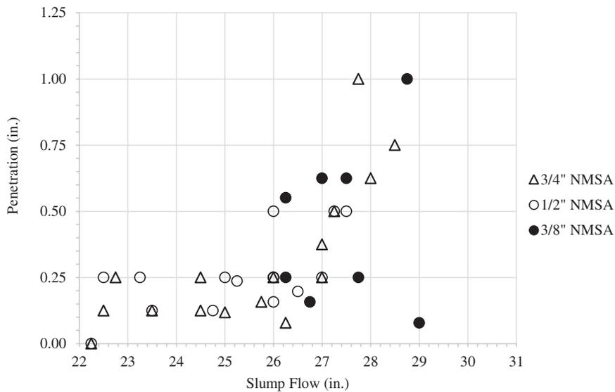
Figure 2-6. Penetration versus slump flow.
