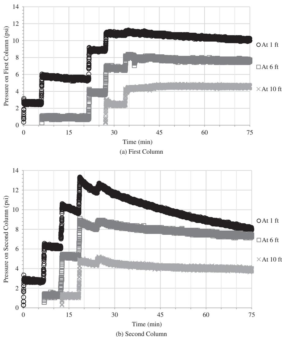
**Figure 2-37. Measured SCC formwork pressure versus time for the two pier columns.**
