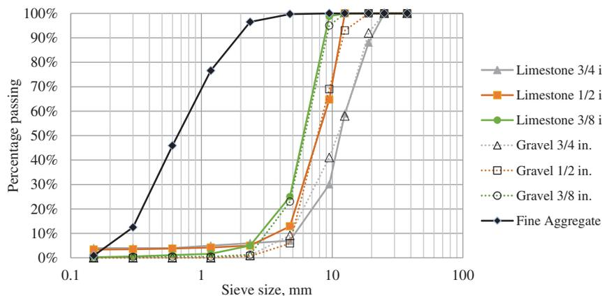
Figure 1-2. Particle size distribution of fine and coarse aggregates.
