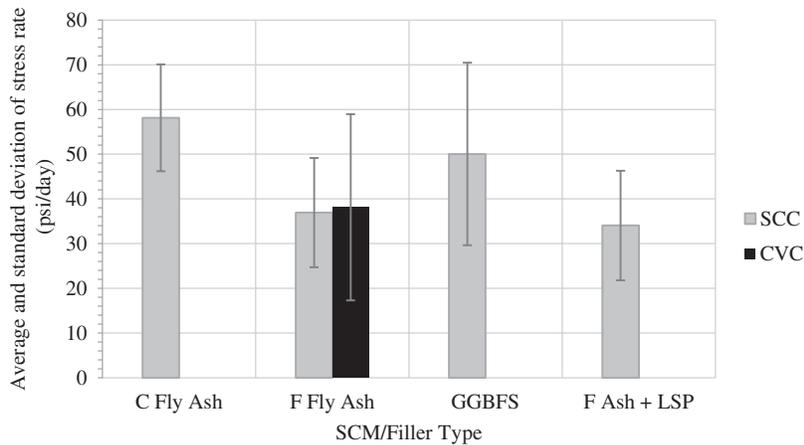
**Figure 2-32. Average and standard deviation of stress rate for CVC and SCC mixtures with different types of SCM/filler.**
