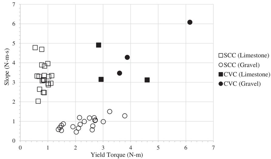
**Figure 2-2. Rheological properties of concrete mixtures.**
