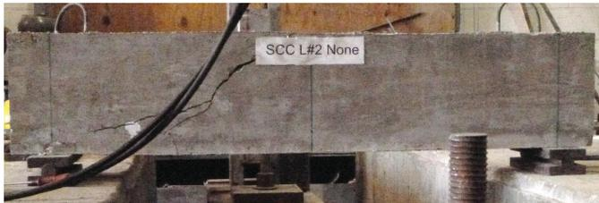
(b) Shear cracking in a low slump flow SCC beam.
