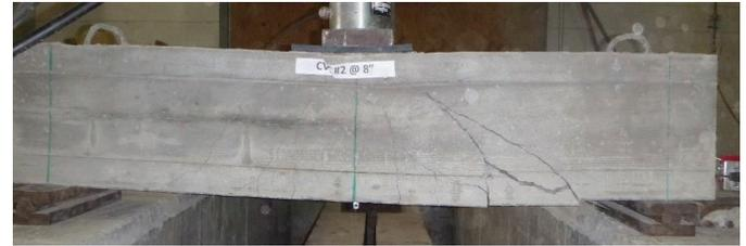
(a) Shear cracking in a CVC beam.
