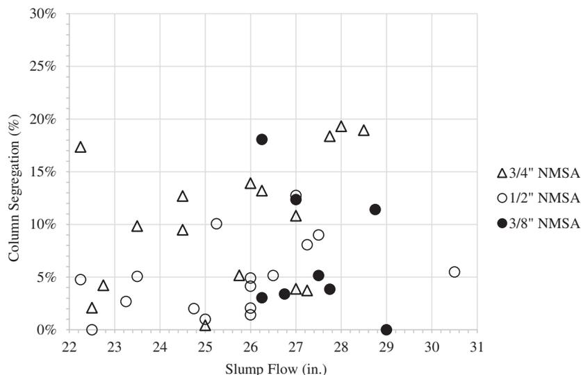
Figure 2-7. Column segregation versus slump flow.
