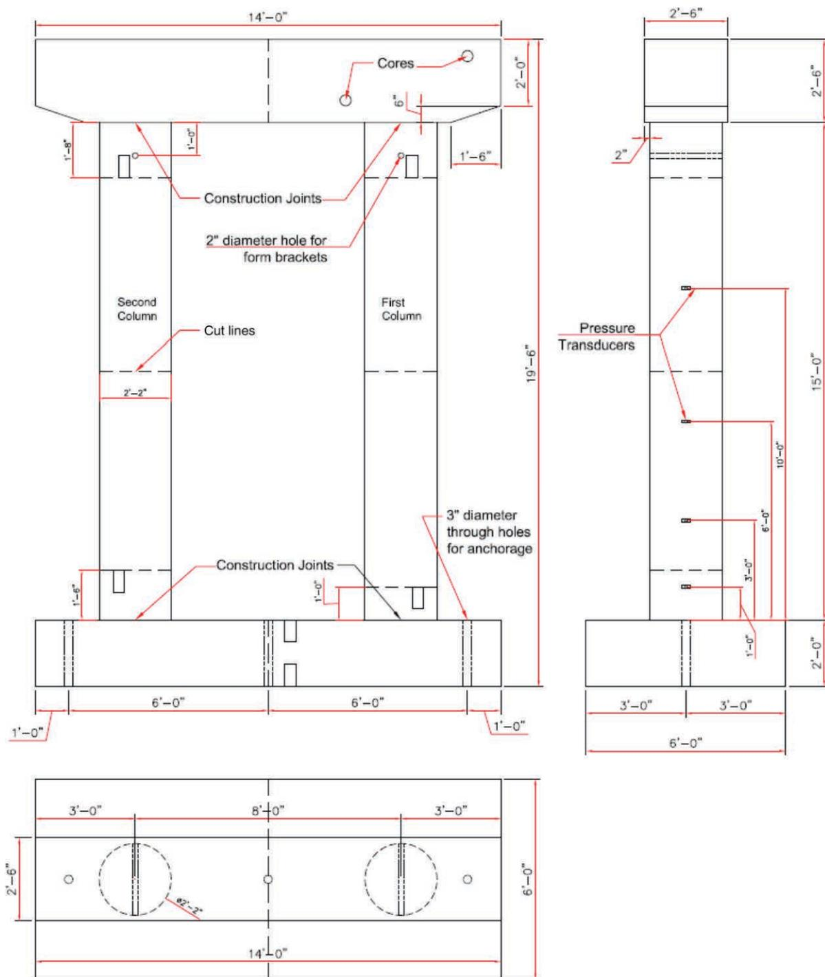
Figure 1-14. Views of the bridge pier specimen.
