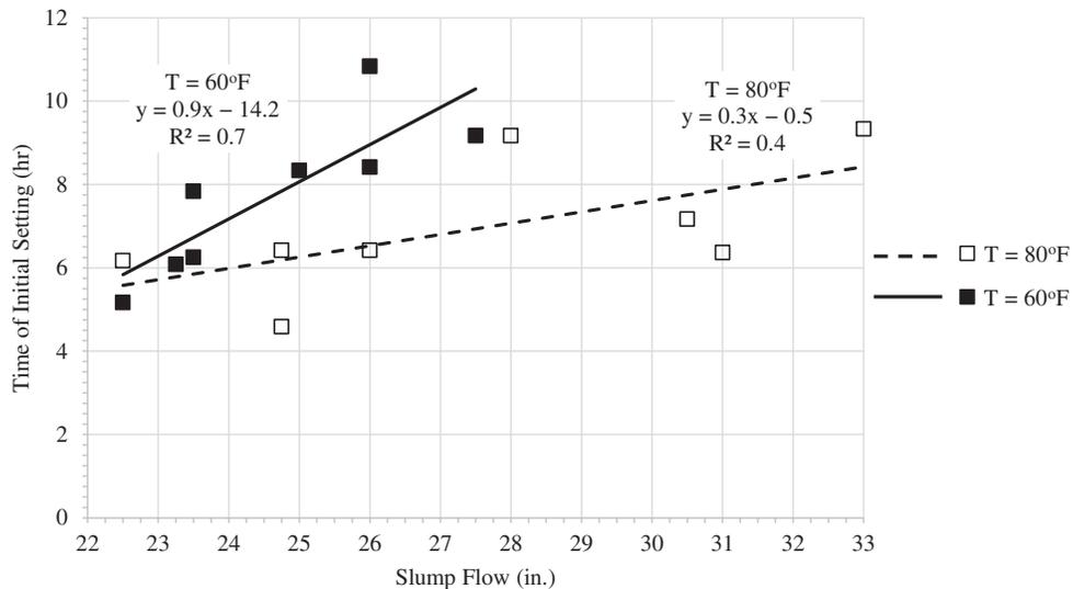
**Figure 2-14. Time of initial setting versus slump flow for SCC mixtures.**
