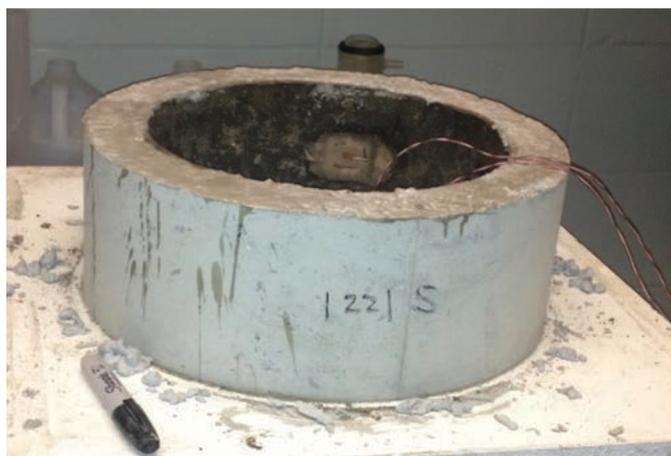
**Figure 1-12. Restrained shrinkage specimen.**
