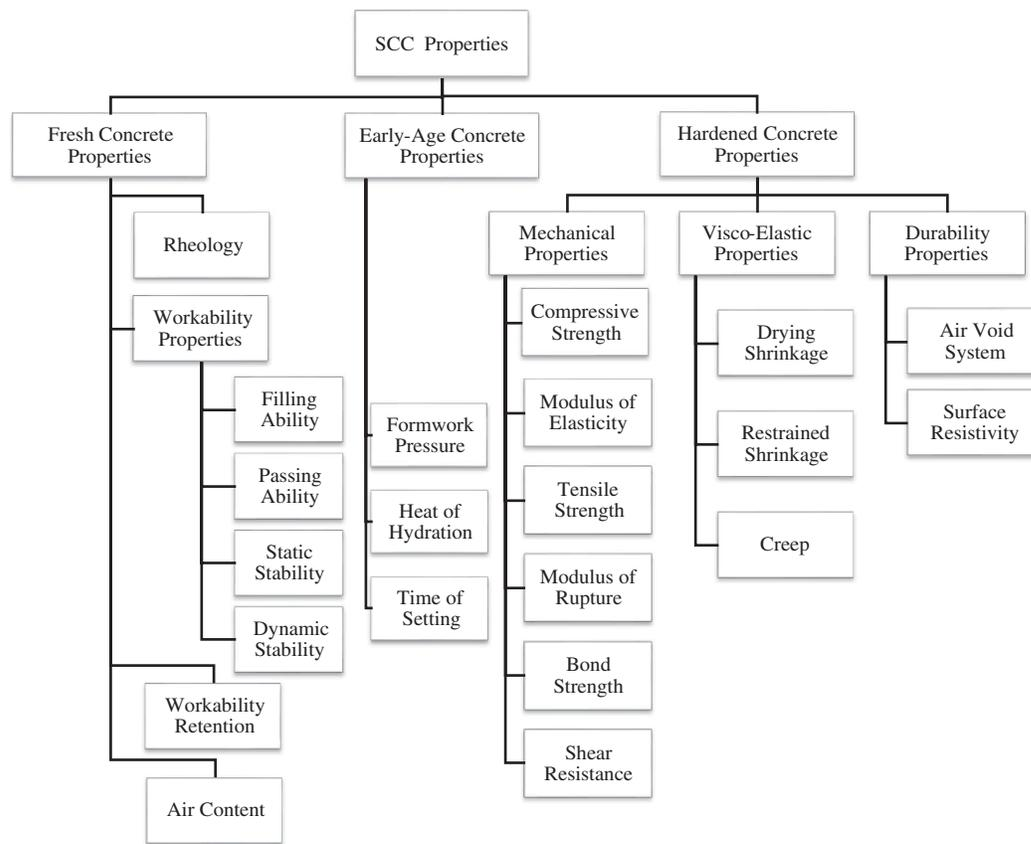
Figure 1-1. SCC properties considered in the experimental investigation.
