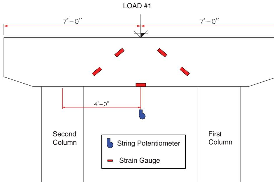
**Figure 1-18. Pier cap test setup.**
