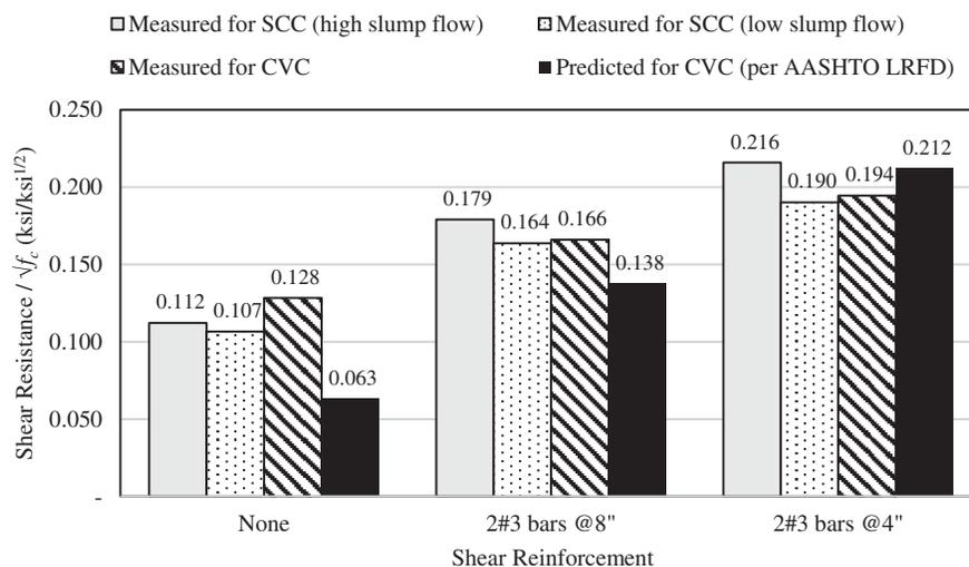
**Figure 2-26. Shear resistance of SCC and CVC mixtures with different reinforcement.**
