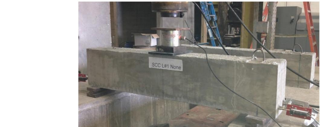
Figure 1-10. Beam shear test setup.
