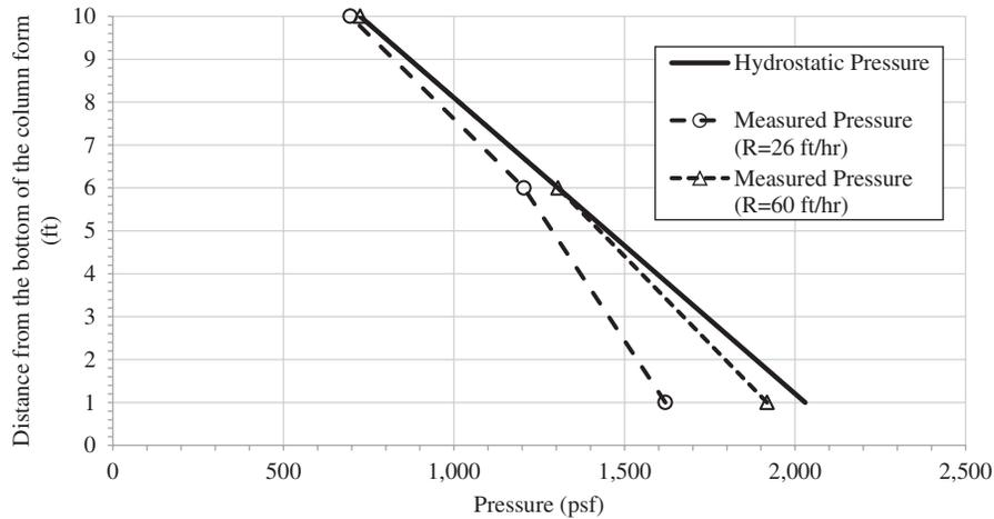
**Figure 2-38. Measured SCC formwork peak pressure for different placement rates.**
