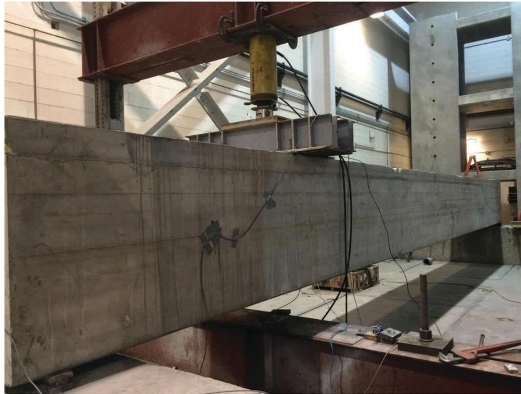
Figure 1-21. Setup of the shear test of box girder specimen.
