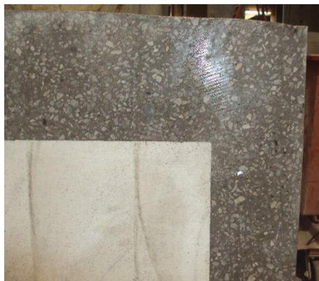
**Figure 2-44.** Saw cut in the bridge box girder specimen showing top and bottom corners.
