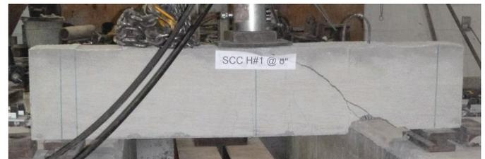
(c) Shear cracking in a high slump flow SCC beam.
