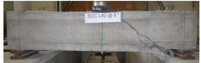
(b) Shear cracking in a low slump flow SCC beam.
