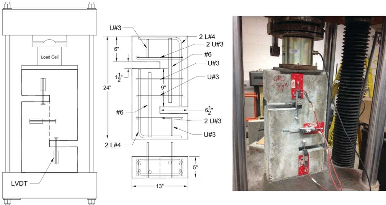
Figure 1-9. Push-off test setup.
