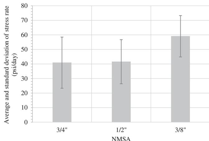
**Figure 2-33. Average and standard deviation of stress rate for SCC mixtures with different NMSA.**
