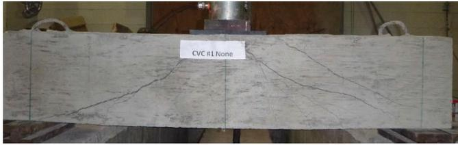
(a) Shear cracking in a CVC beam.
