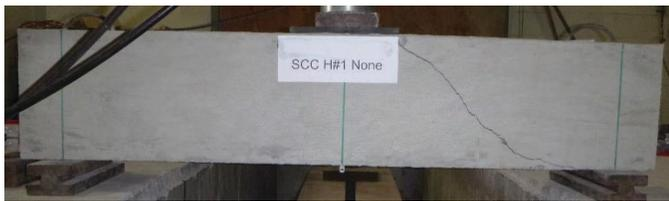
(c) Shear cracking in a high slump flow SCC beam.
