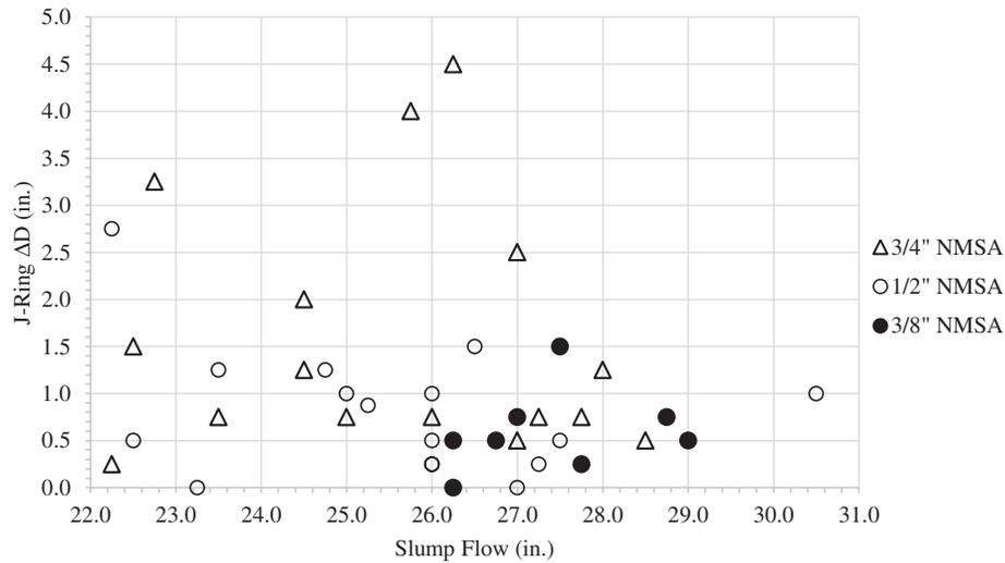
**Figure 2-3. J-ring reduction in slump flow diameter ( $\Delta D$ ) of SCC versus slump flow.**
