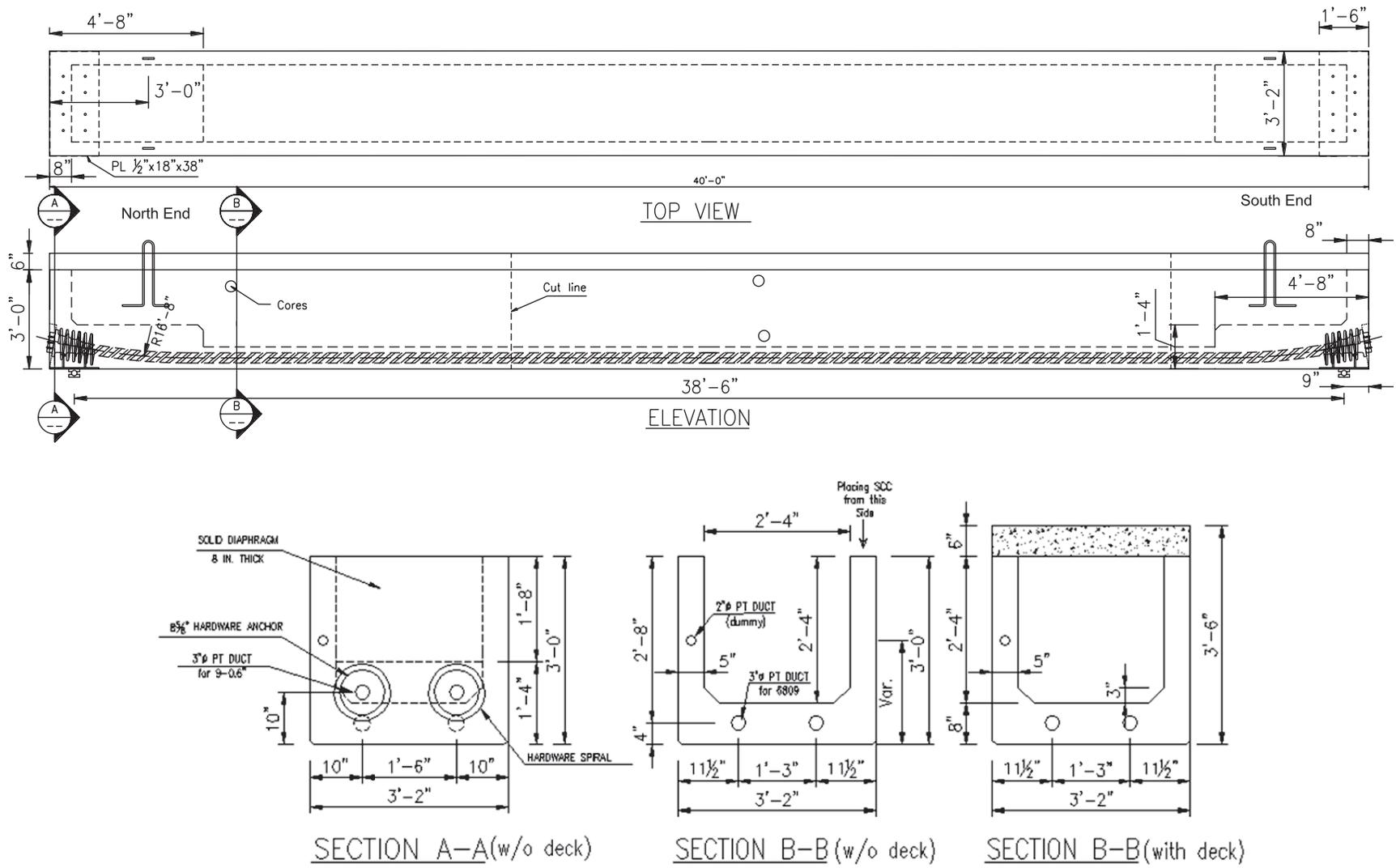
Figure 1-16. Views of the bridge post-tensioned box girder specimen.
