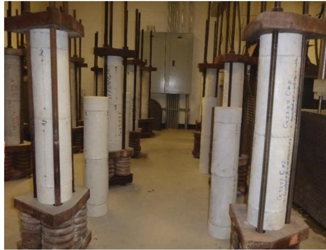
Figure 1-13. Creep test setup.
