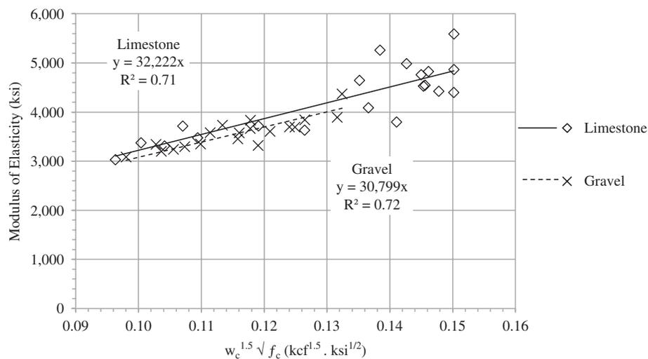
**Figure 2-16. Comparing MOE of SCC mixtures containing gravel and limestone aggregates.**
