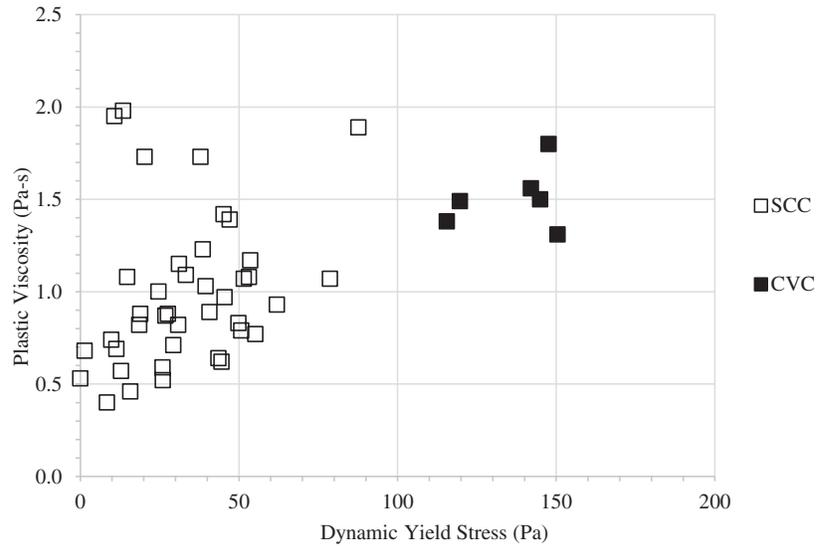
**Figure 2-1. Rheological properties of mortar mixtures.**
