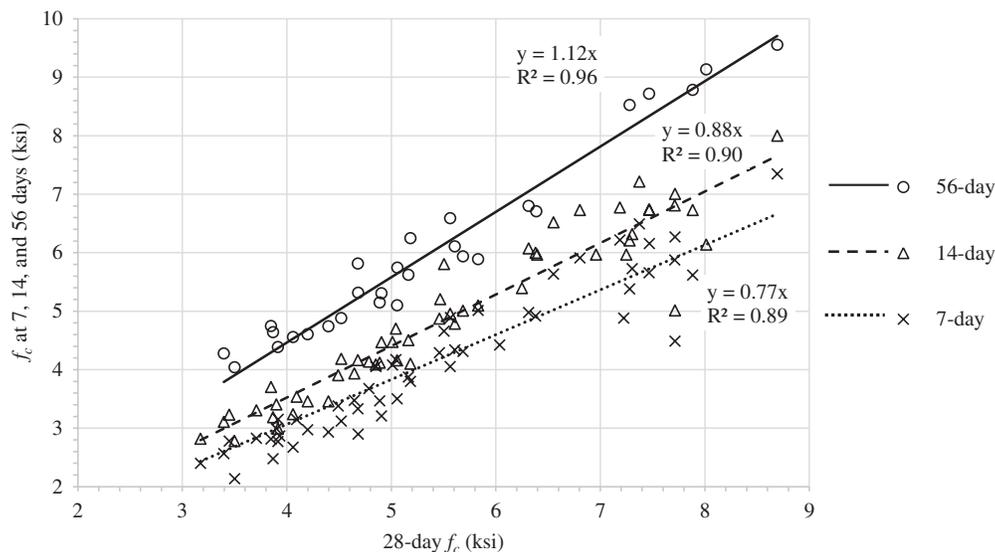
**Figure 2-15. Relationships between average compressive strength at 7, 14, and 56 days and average compressive strength at 28 days for SCC mixtures.**
