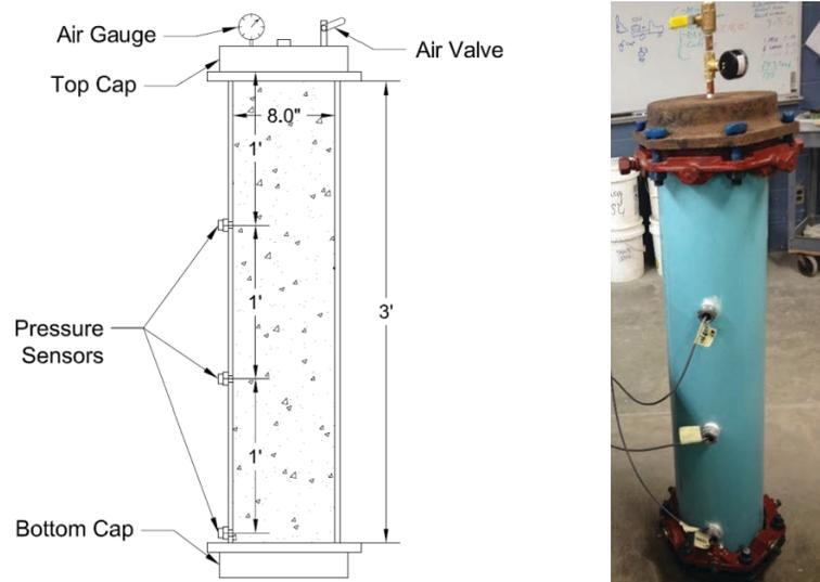
Figure 1-6. Form pressure device.
