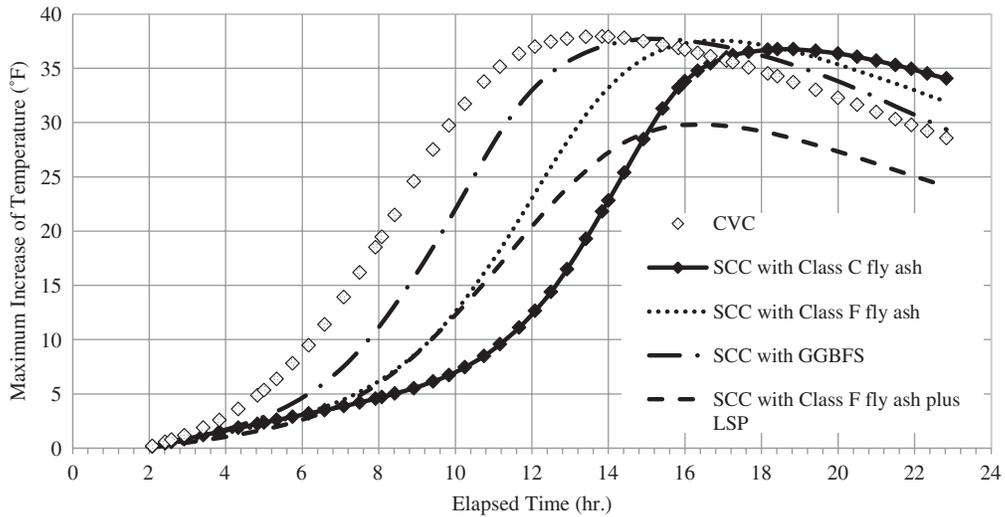
**Figure 2-12. Semi-adiabatic calorimetry test results for mixtures containing 1/2 in. nominal maximum size limestone aggregates.**
