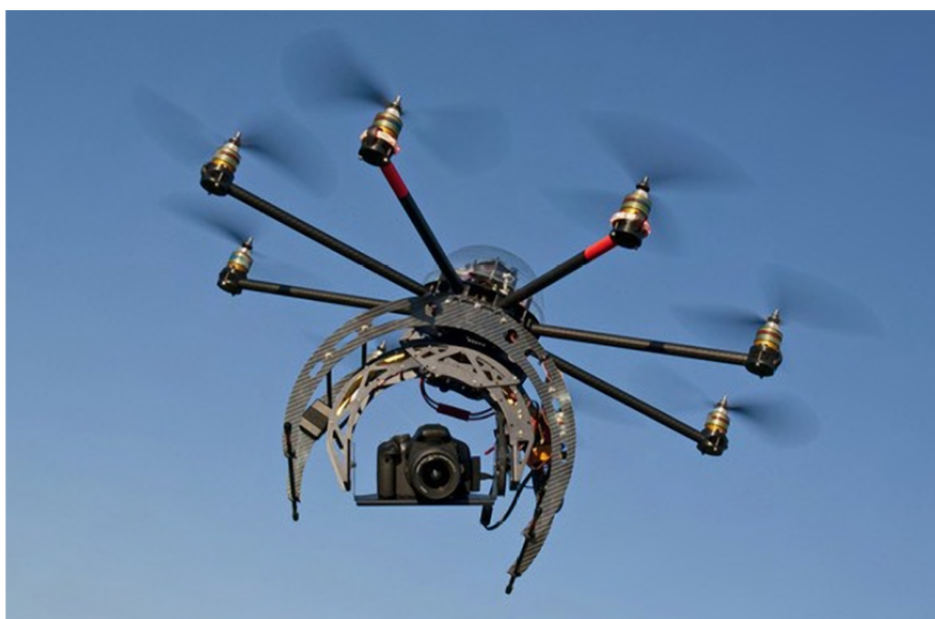
FIGURE 3.2 UAV with an off-the-shelf camera attached. (Source: Fast Company.)
