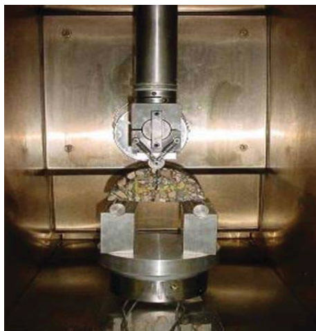
Semi circular bend test set up
