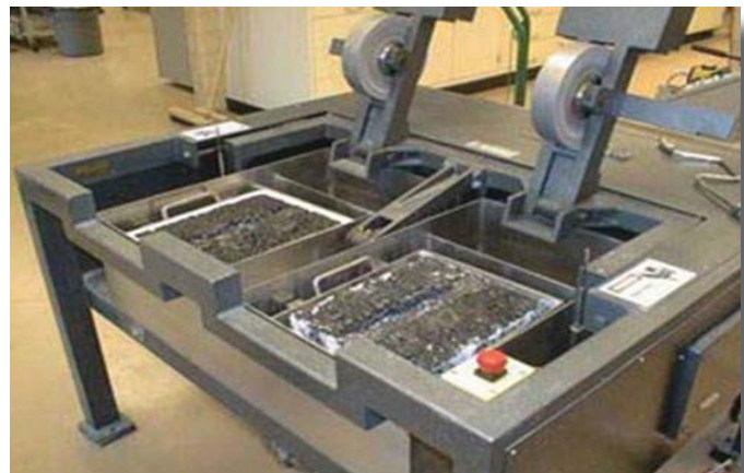
Loaded wheel tracking test set up
