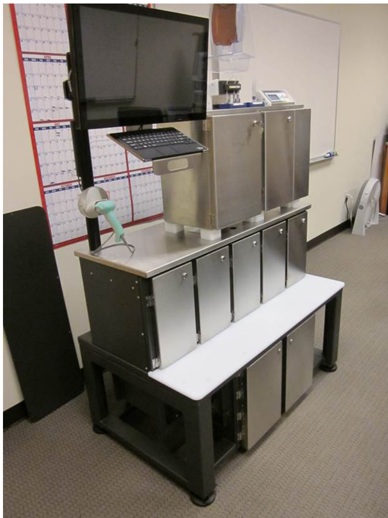
FIGURE 4.4 NorthStar's RadioGenix Tc-99m Generating System. The system is 54" (1.4 m) wide × 28" (0.7 m) deep × 75" (1.9 m) tall, including the monitor. SOURCE: Jim Harvey, NorthStar Medical Radioisotopes.
