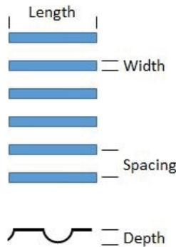
FIGURE 5 Shoulder rumble strip dimensions referenced.
