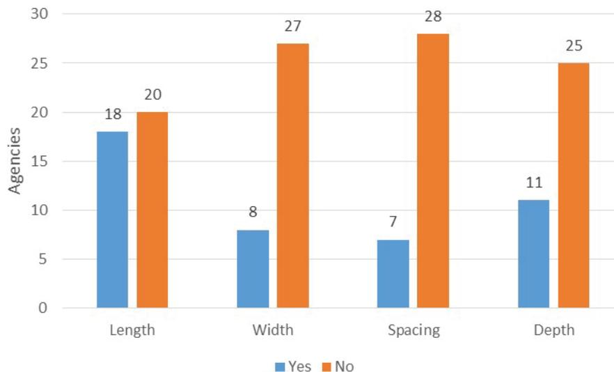
FIGURE 6 Do shoulder rumble strip dimensions vary by roadway type (survey question 23)?
