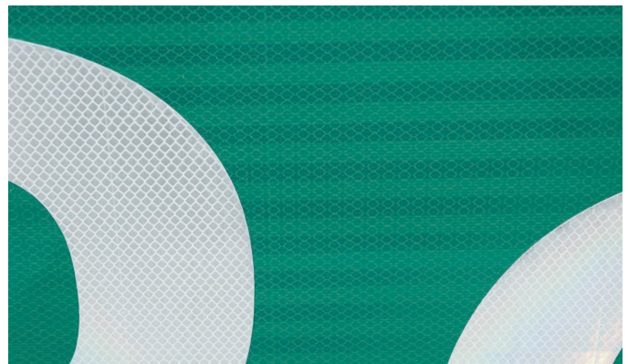
Figure 7. Type XI prismatic legend on Type IV prismatic background.
