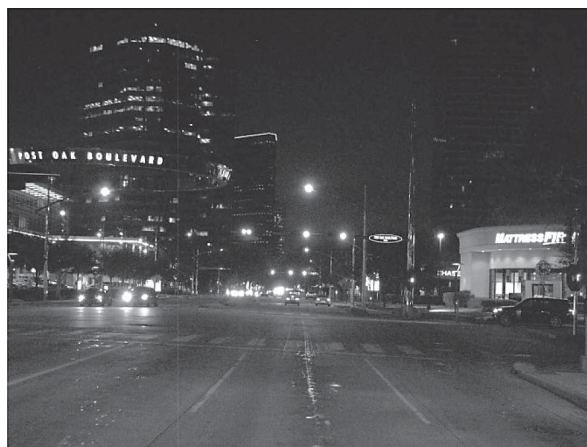
Level 4 Visual Complexity: Moderate commercial and roadway lighting. Several illuminated objects in view. Moderate traffic.
