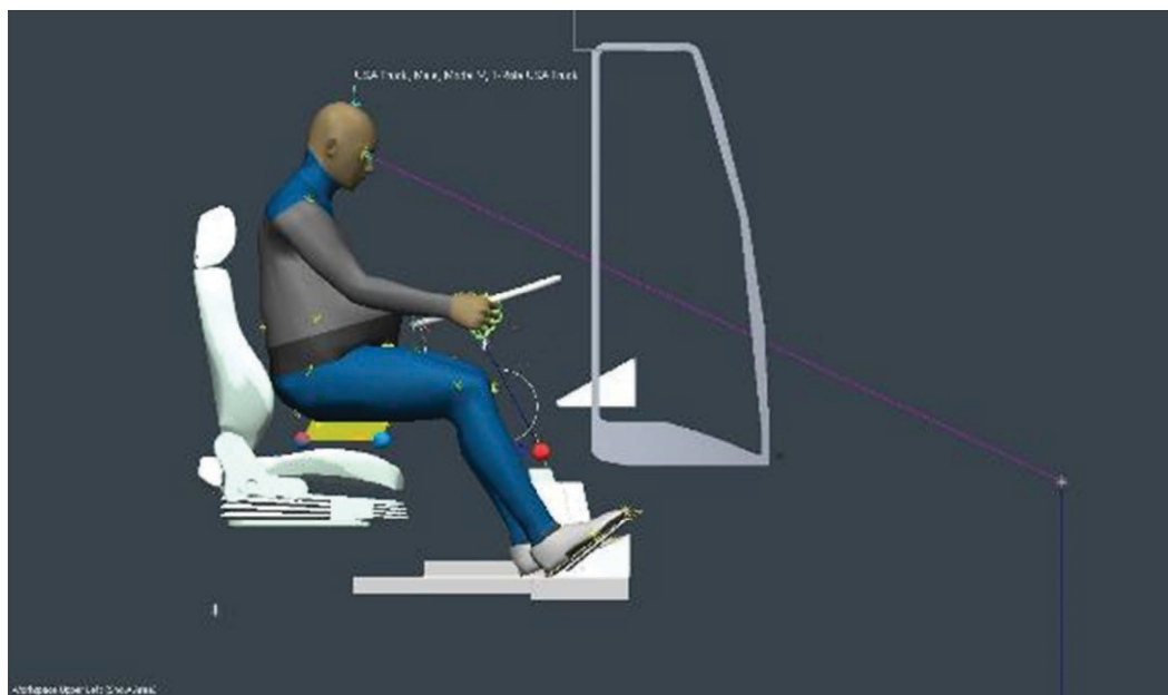
Figure 27. SAE shin/knee contours and stomach contour near manikin Male V (red-dotted curves).
