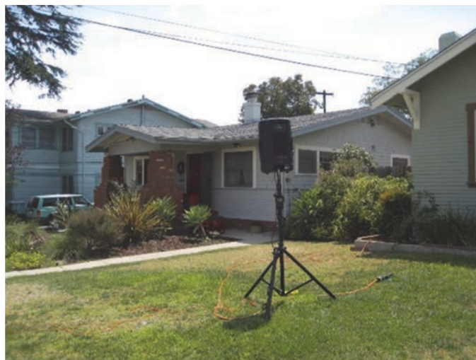
Figure 4-3. Ground-level loudspeaker measurement in San Diego.
