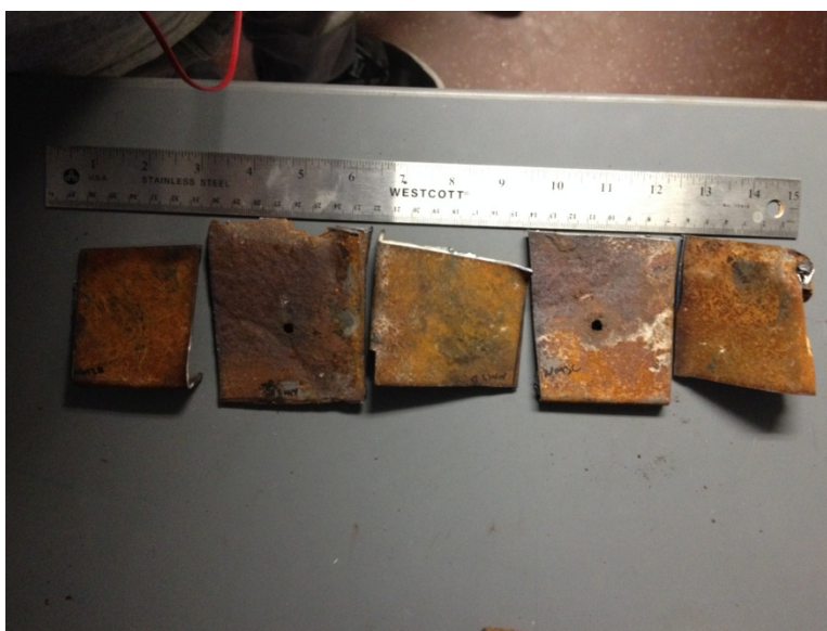
Figure 20 Samples NM3 used in corrosion study.
