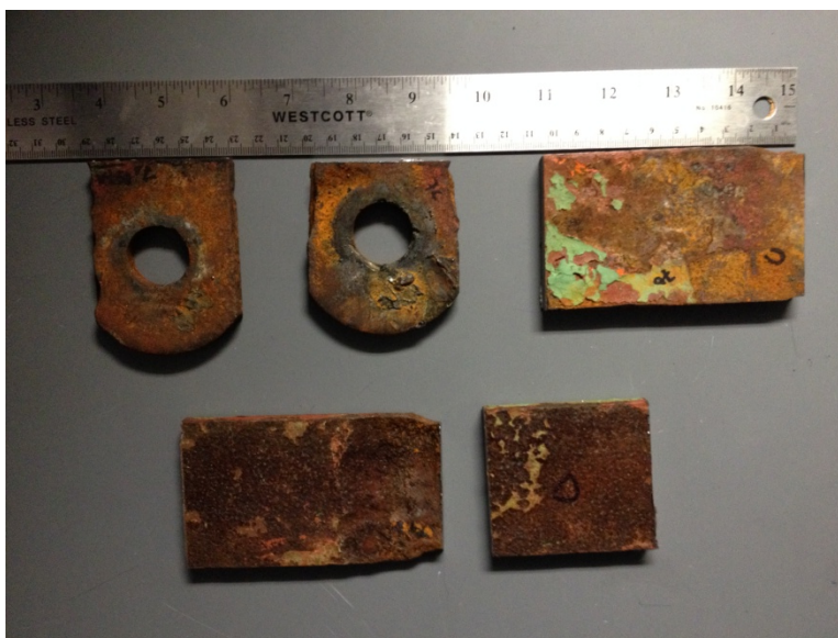
Figure 18 Corrosion samples used from the Brightman Street Bridge.
