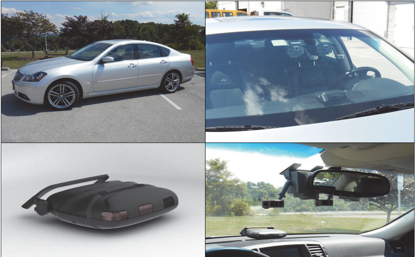
Figure 2.2. M35 (upper left), outside view of the two head units and MiniDAS (upper right), MiniDAS (lower left), and inside view of two head units and MiniDAS (lower right).
