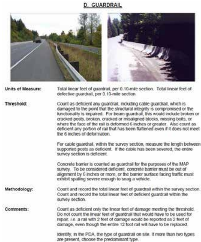
FIGURE 3 Sample rating instructions for guardrail under a scored system (WSDOT 2014).
