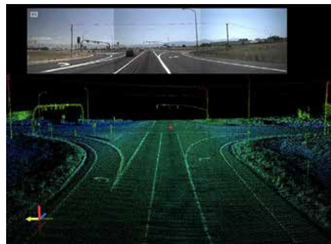
FIGURE 4 Example use of LiDAR to roadway asset inventory (Ellsworth 2014).
