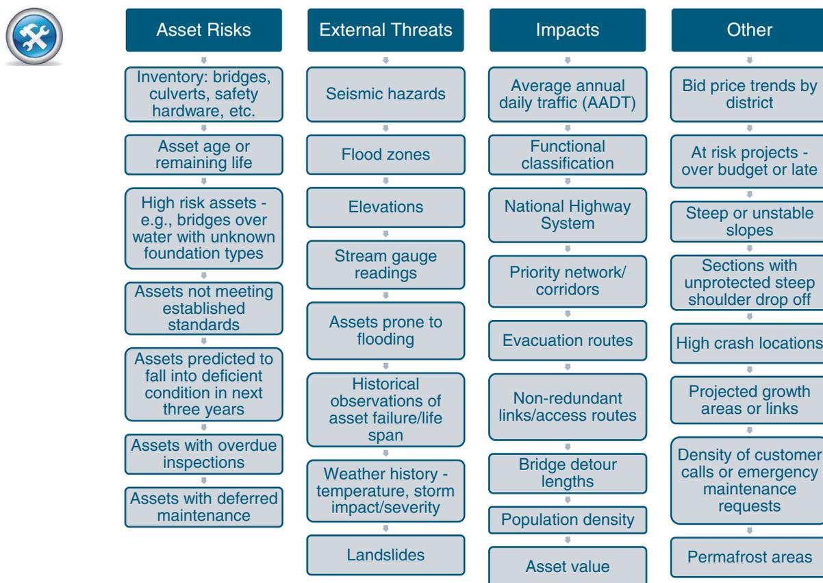
**Figure 7. Using GIS to Assess and Manage Risks—Sample Data Layers**
