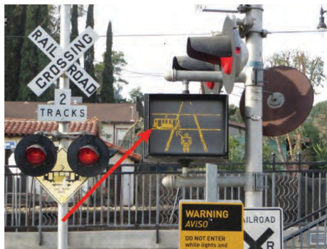
Figure 90. The pictogram within this blank-out sign in Los Angeles shows a side view of trains approaching from the left.
