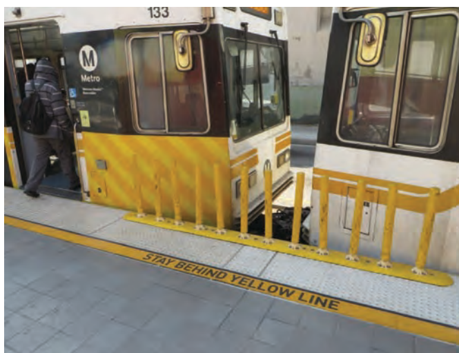
Figure 40. Flexible delineators as between-car barriers to prevent passengers who are blind from falling between rail cars.
