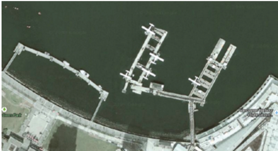
FIGURE 17 Typical H-dock layout design at Vancouver Seaplane Terminal, British Columbia. (Source: Google maps, Digitglobal, IMTCAN, Province of British Columbia)
