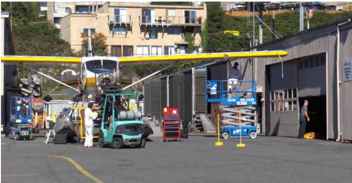
FIGURE 12 Maintenance being performed outdoors on a float seaplane. (Credit: S. Quilty, SMQ Airport Services)
