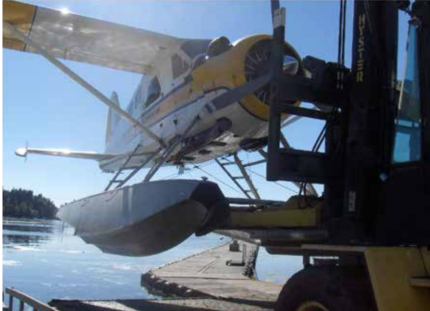
FIGURE 11 Aircraft lifted from rail system with forklift attachment. (Credit: S. Quilty, SMQ Airport Services)
