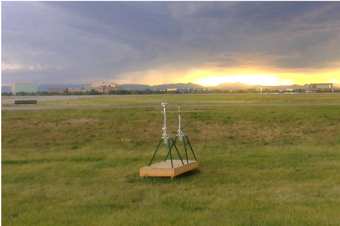
Figure 7 BGI PQ100 PM samplers for PM_{2.5} ( PM_{10} inlet followed by a PM_{2.5} cyclone) (left) and TSP inlet (right)
