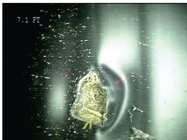
FIGURE 13 Approximately 2-in.-diameter puncture in HDPE pipe.
