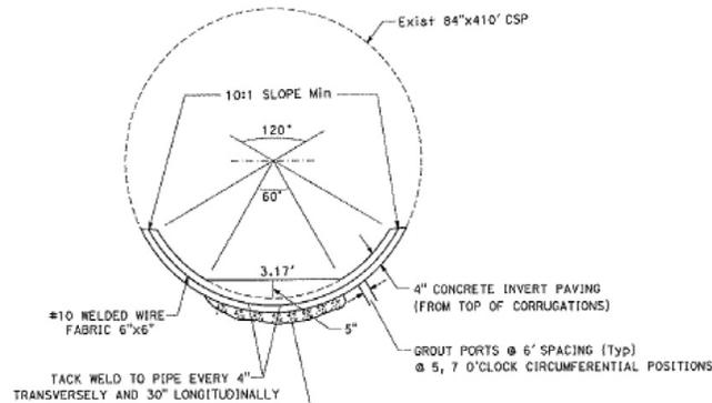
FIGURE 28 Standard detail for concrete invert paving (Caltrans 2013).
