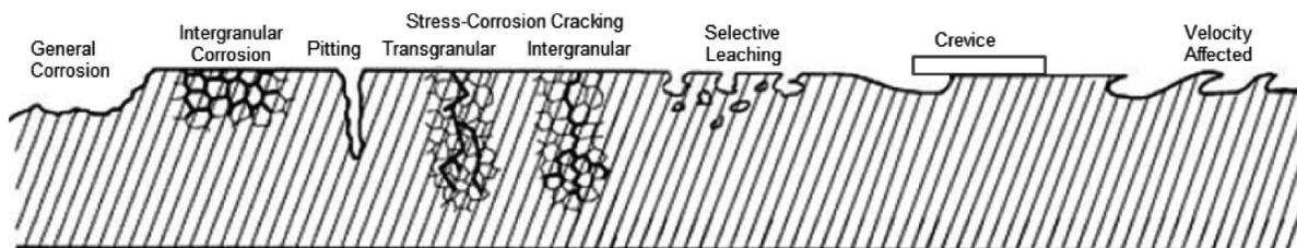
FIGURE 8 Table and schematics of common corrosion mechanisms (after ASM International 2003).
