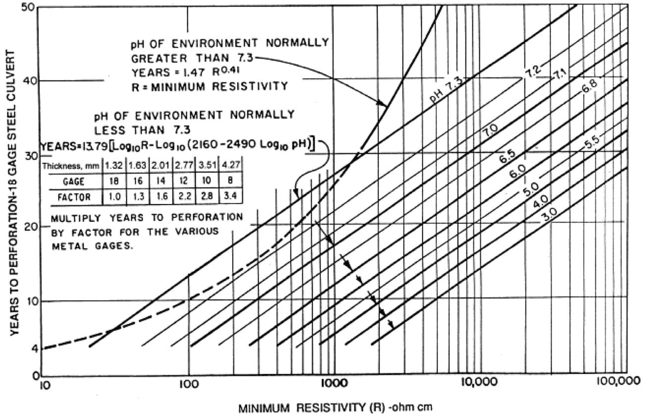
FIGURE B2 Chart for estimating years to perforation of steel culverts using California method (Caltrans 1999).
