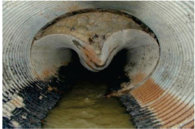
FIGURE 36 Failed culvert under I-480 in 2001 (FHWA 2014).
