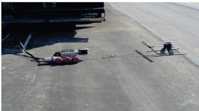
FIGURE 35 Laser profiler and CCTV used in tandem for pipe inspections.
