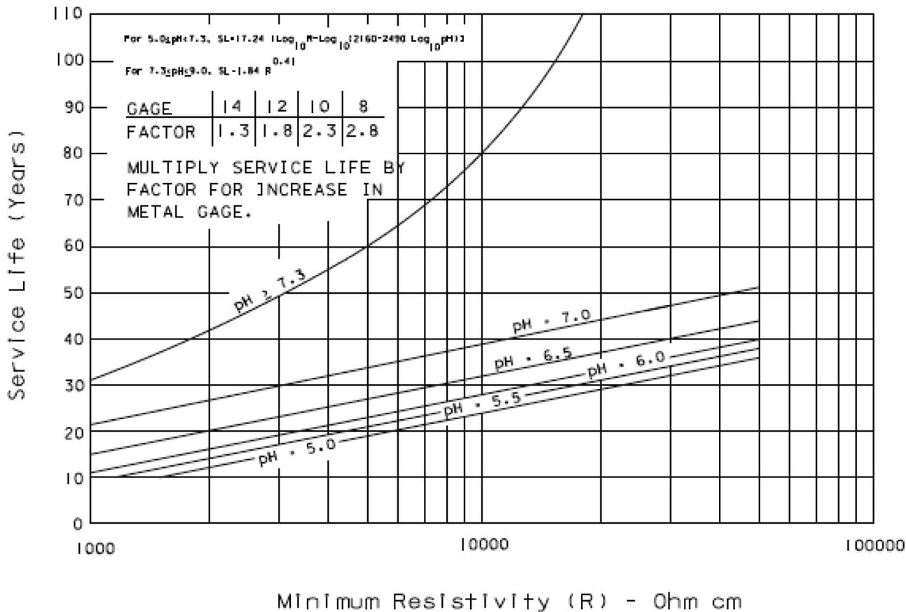
FIGURE B5 Estimated service life versus pH and resistivity for 16-gage galvanized steel using FDOT method (FDOT 2012).
