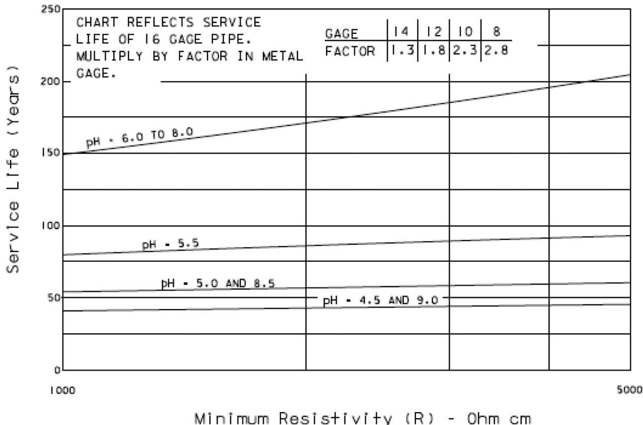
FIGURE B8 Estimated service life versus pH and resistivity for aluminum using FDOT method (FDOT 2012).
