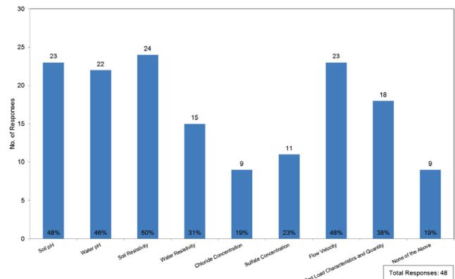
FIGURE 4 Types of environmental parameters collected for MSL evaluations.
