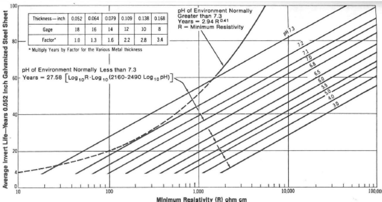
FIGURE B3 Chart for estimating average invert life using AISI method (AISI 1994).
