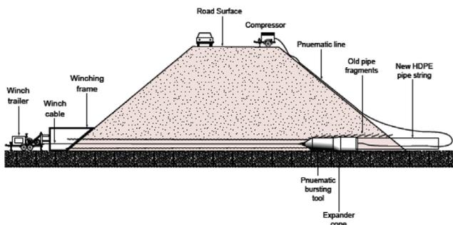
FIGURE 34 Pipe bursting schematic (USDA Forest Service 2005).
