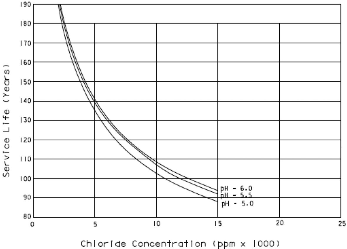
FIGURE B1 Estimated service life versus pH and resistivity for 60-in.-diameter concrete culverts, S = 1,500 ppm (FDOT 2012).
