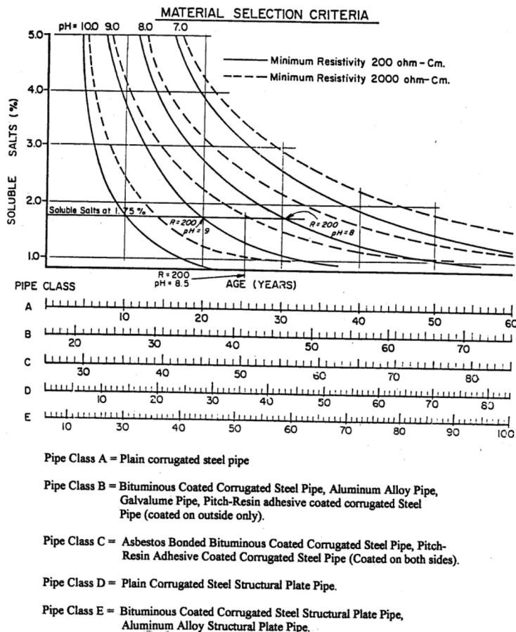
FIGURE B6 Utah DOT material selection criteria for metal pipe (Leatham and Peterson 1977).
