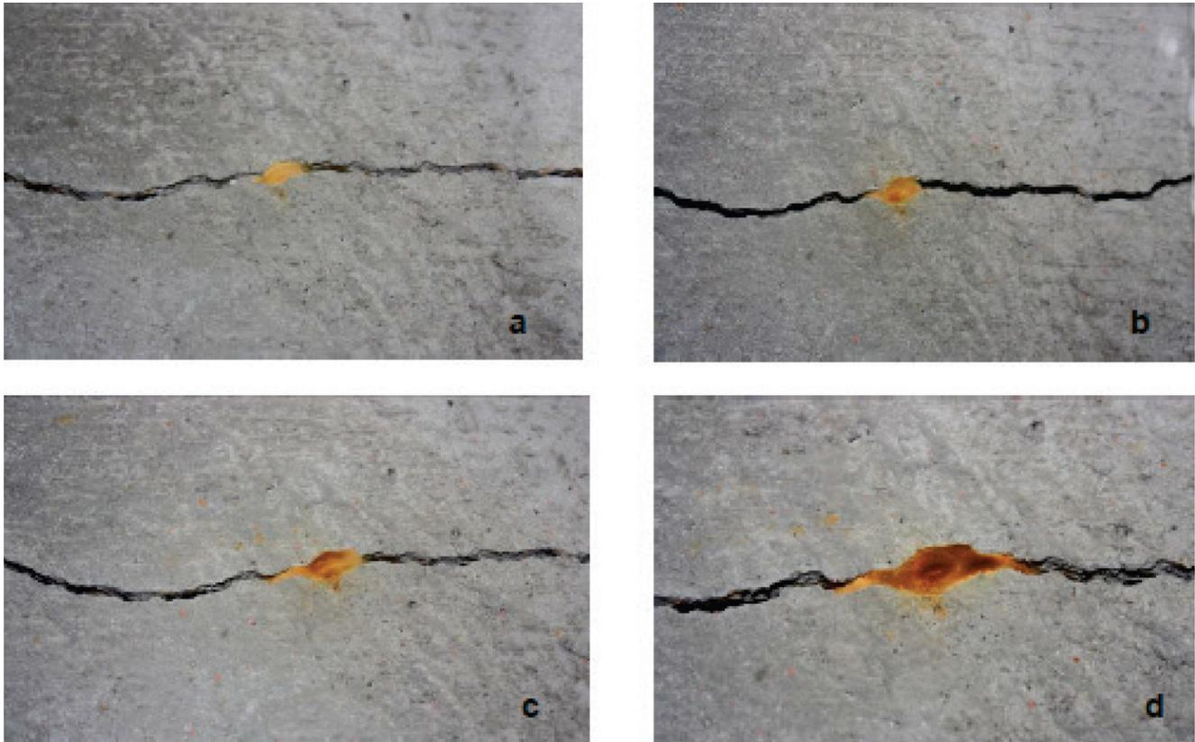
FIGURE 21 Progression of corrosion in RCP with a 0.100-in. crack exposed to chloride solution after (a) 6 days, (b) 20 days, (c) 34 days, and (d) 52 days (Busba et al. 2011).
