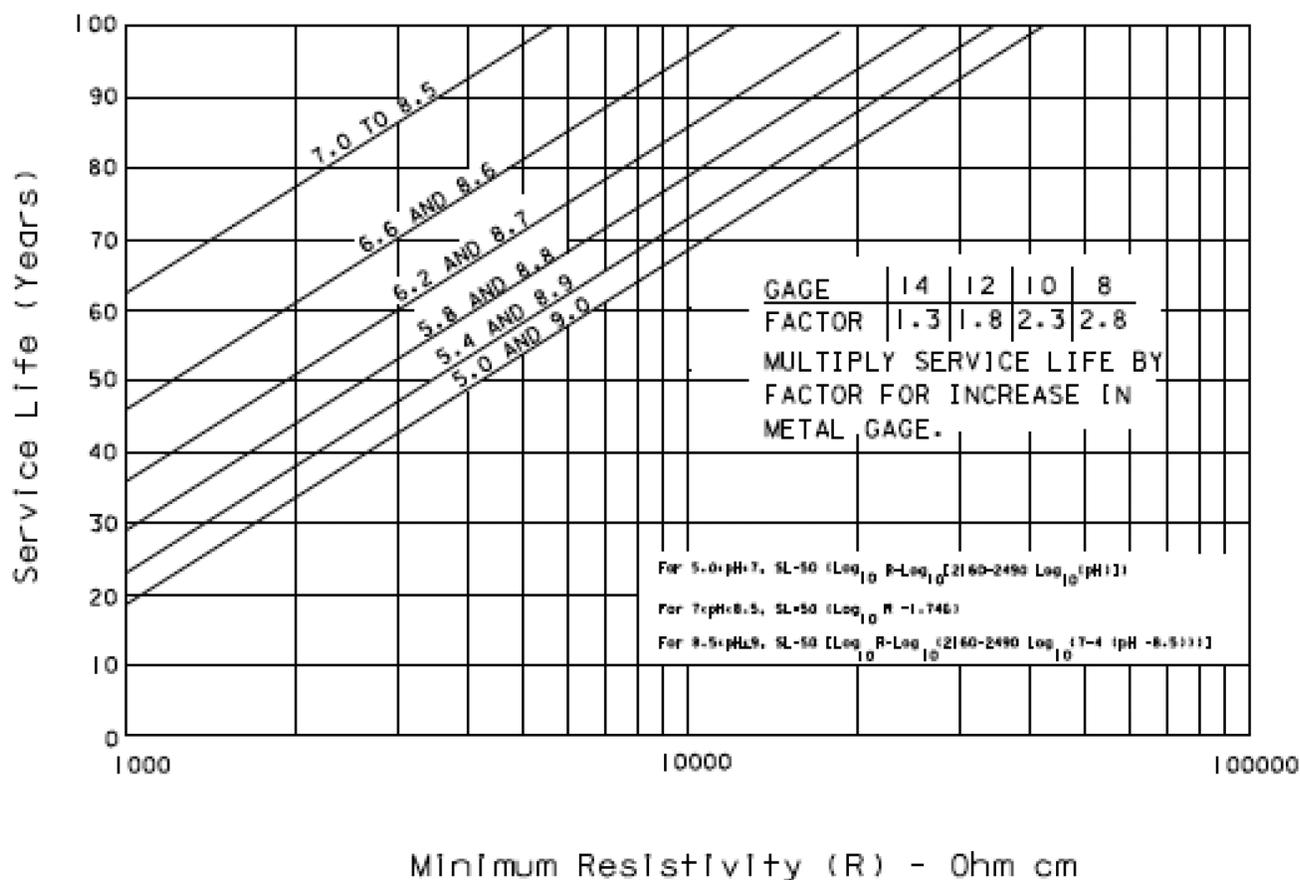
FIGURE B7 Estimated service life versus pH and resistivity for 16-gage aluminized steel type II using FDOT method (FDOT 2012).
