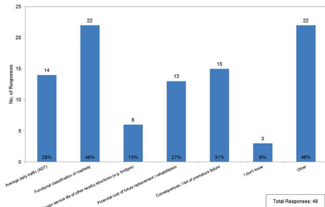
FIGURE 3 Agency bases for determining the design service life of culverts.
