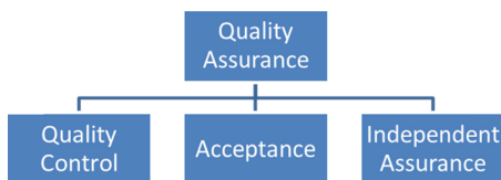
Figure 3. Traditional QA model (Burati et al. 2003).
