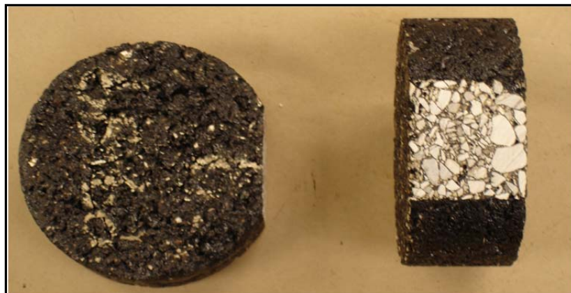
FIGURE 3 Hamburg specimen preparation.
