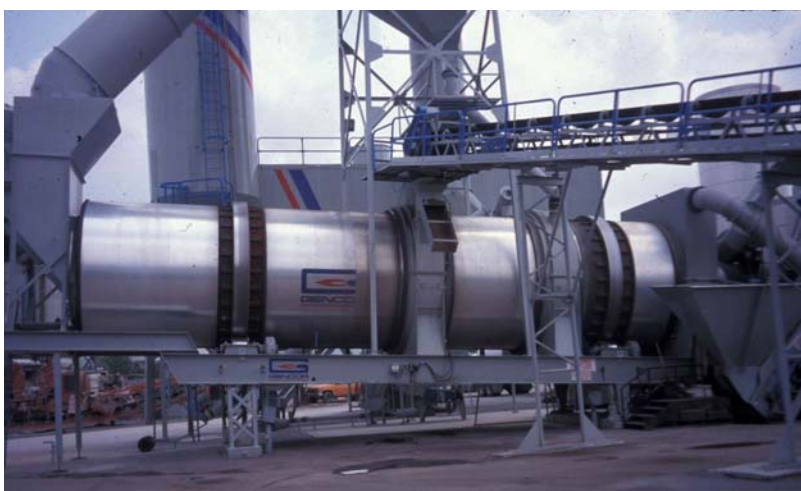
FIGURE 3 Counterflow drum plant illustration.
