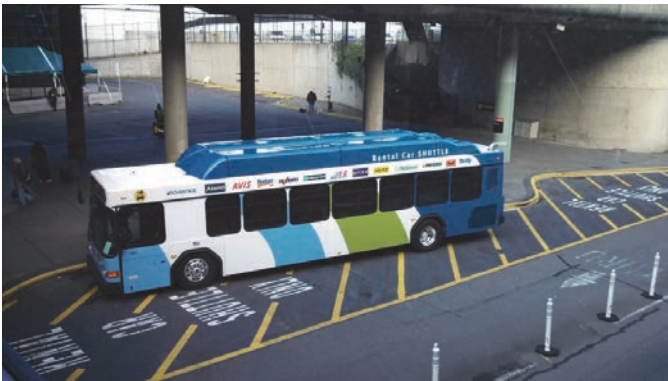
Figure 8-26. Shallow saw tooth boarding spaces at Seattle-Tacoma International Airport.
